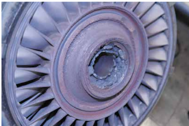
Figure 1 Failed No 7 bearing
