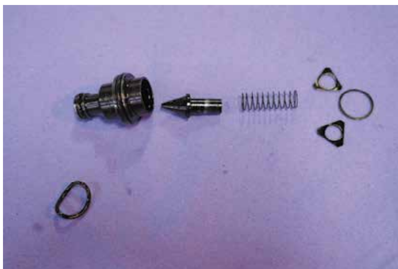
Figure 2 Oil filter housing check valve (disassembled) with foreign O-ring found inside
