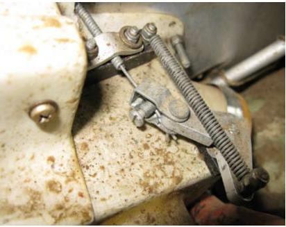
Figure 1 Operating mechanism for engine carburettor heat
