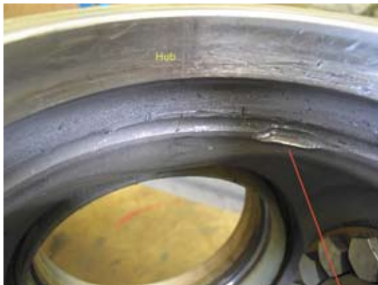
Smear from ball bearing becoming jammed between hub and shank
