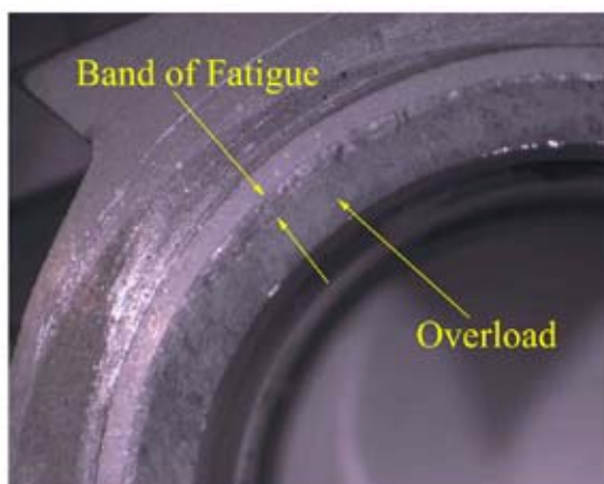
Fracture surface showing narrow fatigue failure and overload region
