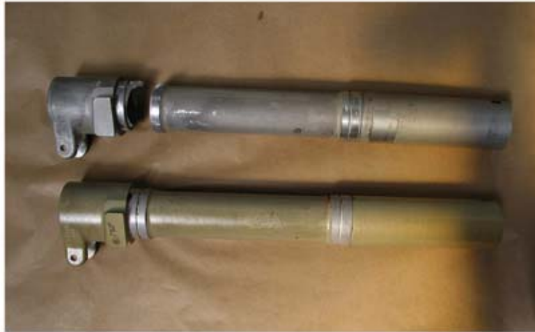
Failed NLG with New NLG
