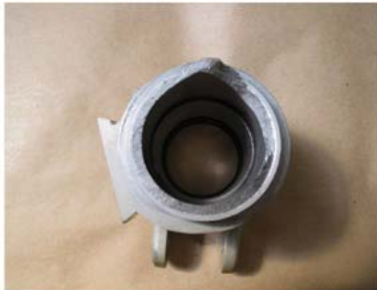
Failed NLG viewed from above
