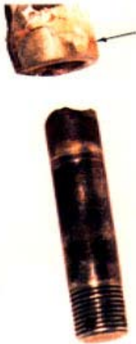
Fig 3. Pivot pin and bottom of strut: separation plane within collar is arrowed. (Photo: HT Consultants)
