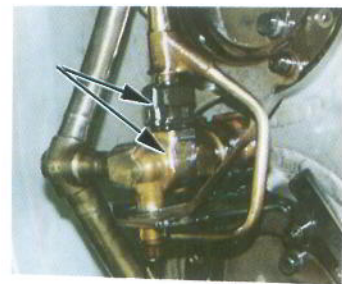
Fig 1a Union nut after tightening to correct torque
