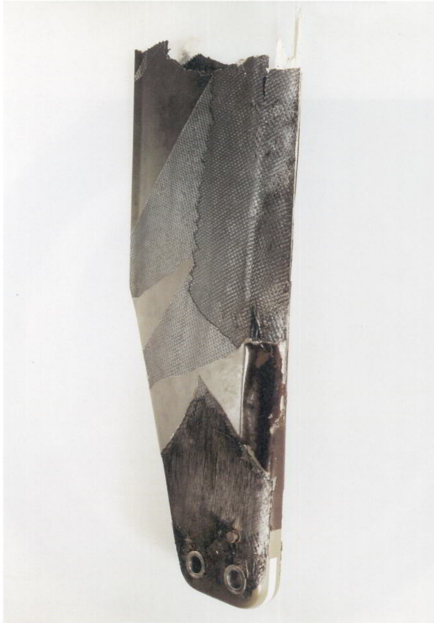
Figure 11: Showing damaged inboard (left) side of 'White' tail rotor blade, with thermal delamination of root area and general delamination outboard, including the leading edge from which the anti-erosion shield detached.
