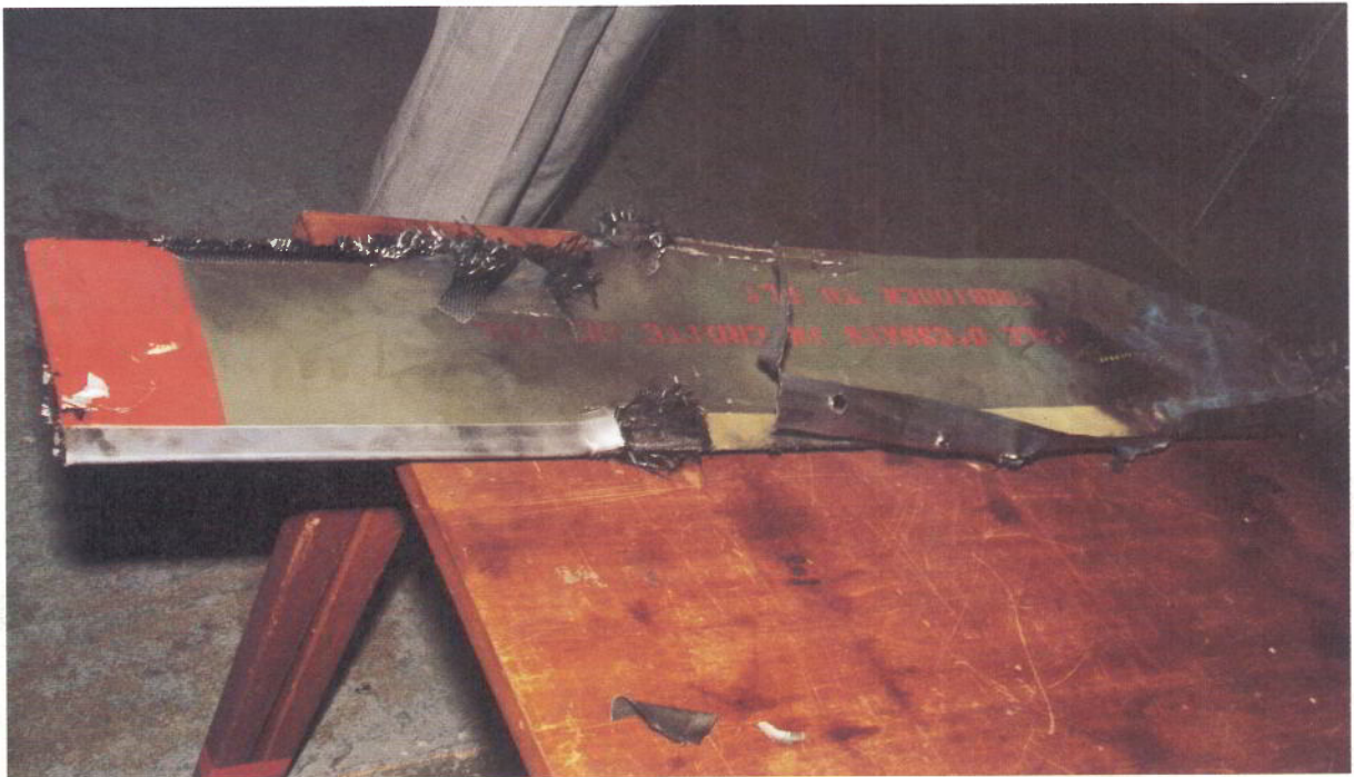
Figure 11B: Showing localised damage to leading edge composite and detached inboard length of shield, with 'burn-holes', on above blade.
