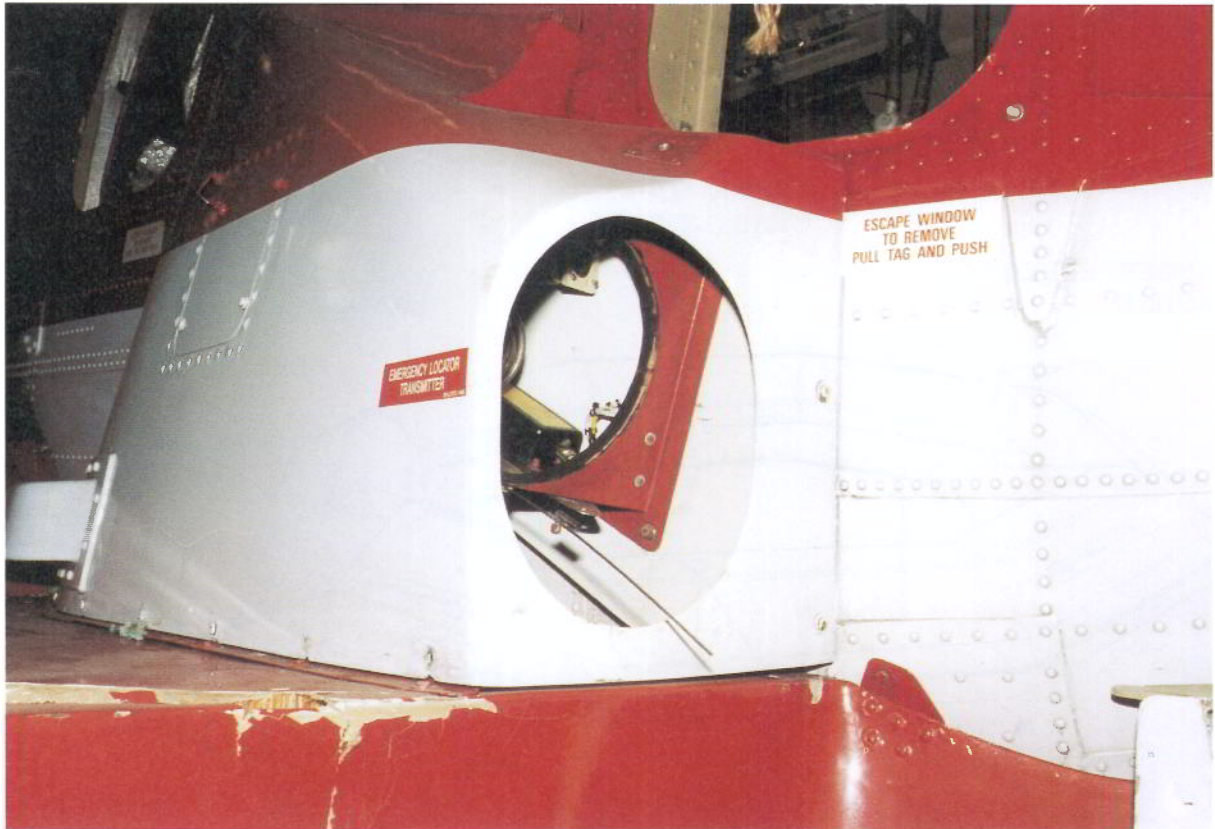
Figure 4: Showing location of the automatically deployable emergency locator transmitter (ADELT) housing.
