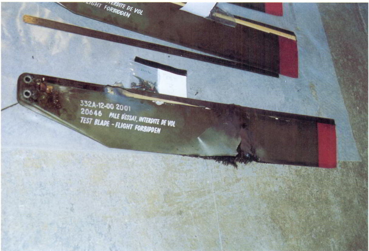
Figure 8A: Showing general marked damage to TRB s/n 20646 after 188.2kA input to trailing edge, 0.5 metre from tip.
