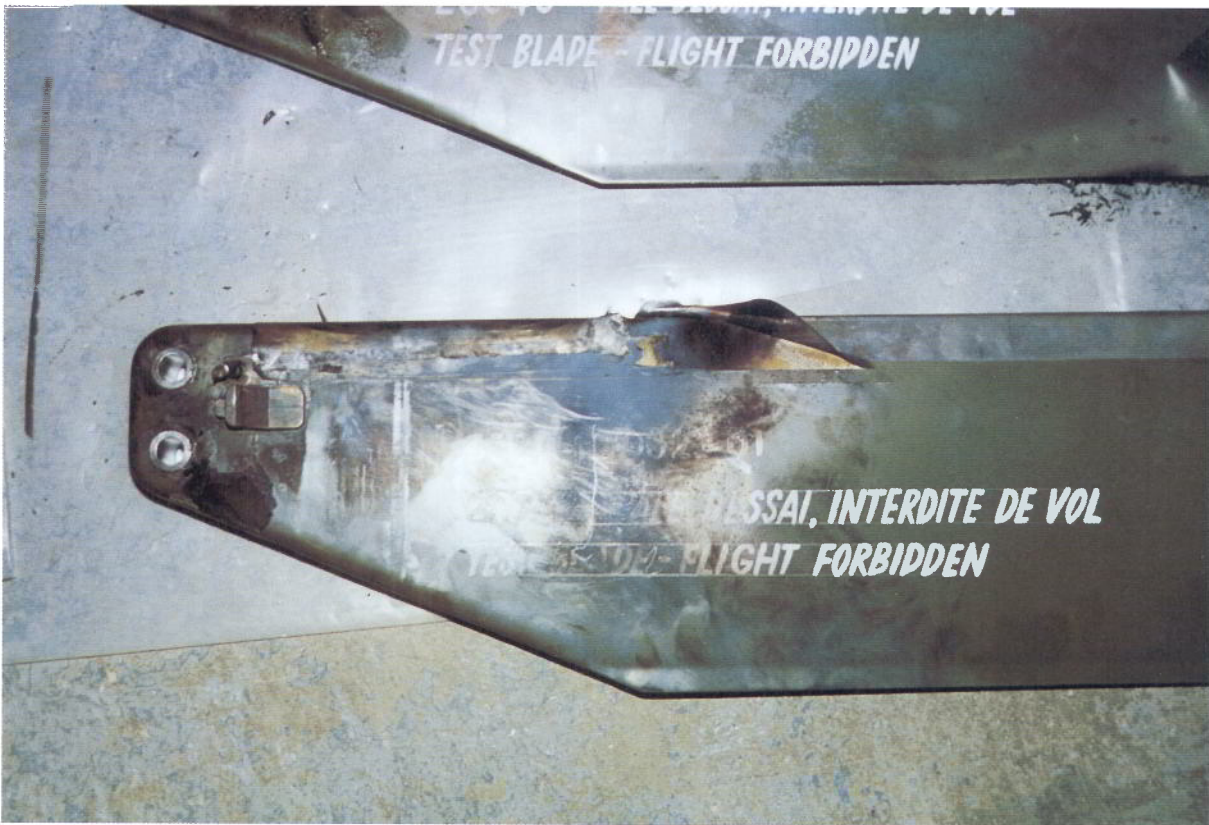
Figure 9A: Showing damage to TRB s/n 20732 after 206.9kA input to inboard end of erosion shield, with local peel-back of shield.
