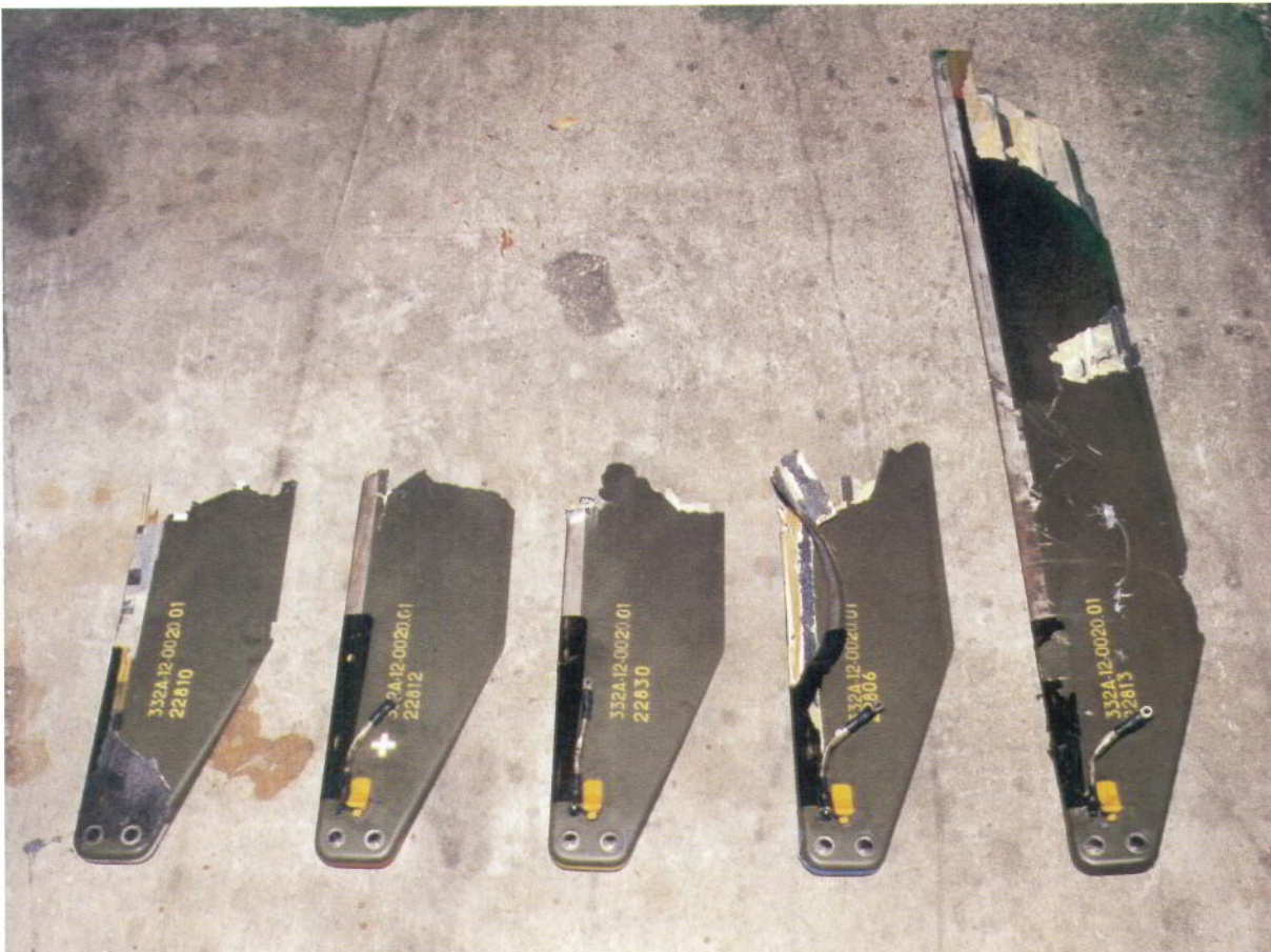
Figure 13: Showing the recovered tail rotor blade sections with, left to right in this photograph, 'White', 'Red', 'Blue' and 'Black' blades, outboard (right) sides uppermost. Note similar lengths of first four severed blades, caused by rotational penetration into aft side of pylon (Figure 5, A-6).
