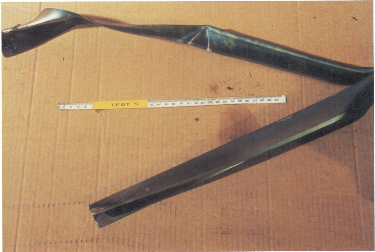
Figure 10A: Showing detached and badly deformed erosion shield after 275.5kA input to aft tip bolt on TRB s/n 20662.
