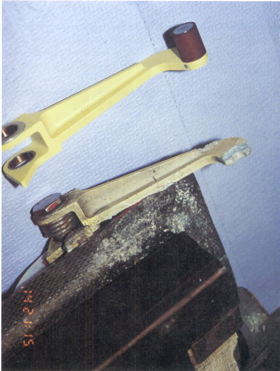
Figure 5: Showing hook-shaped broken end of spring-loaded arm at upper forward corner of left main door, after detachment of roller end, with new arm/roller for comparison; aft arm on this door and forward arm on right door were also broken in this manner.
