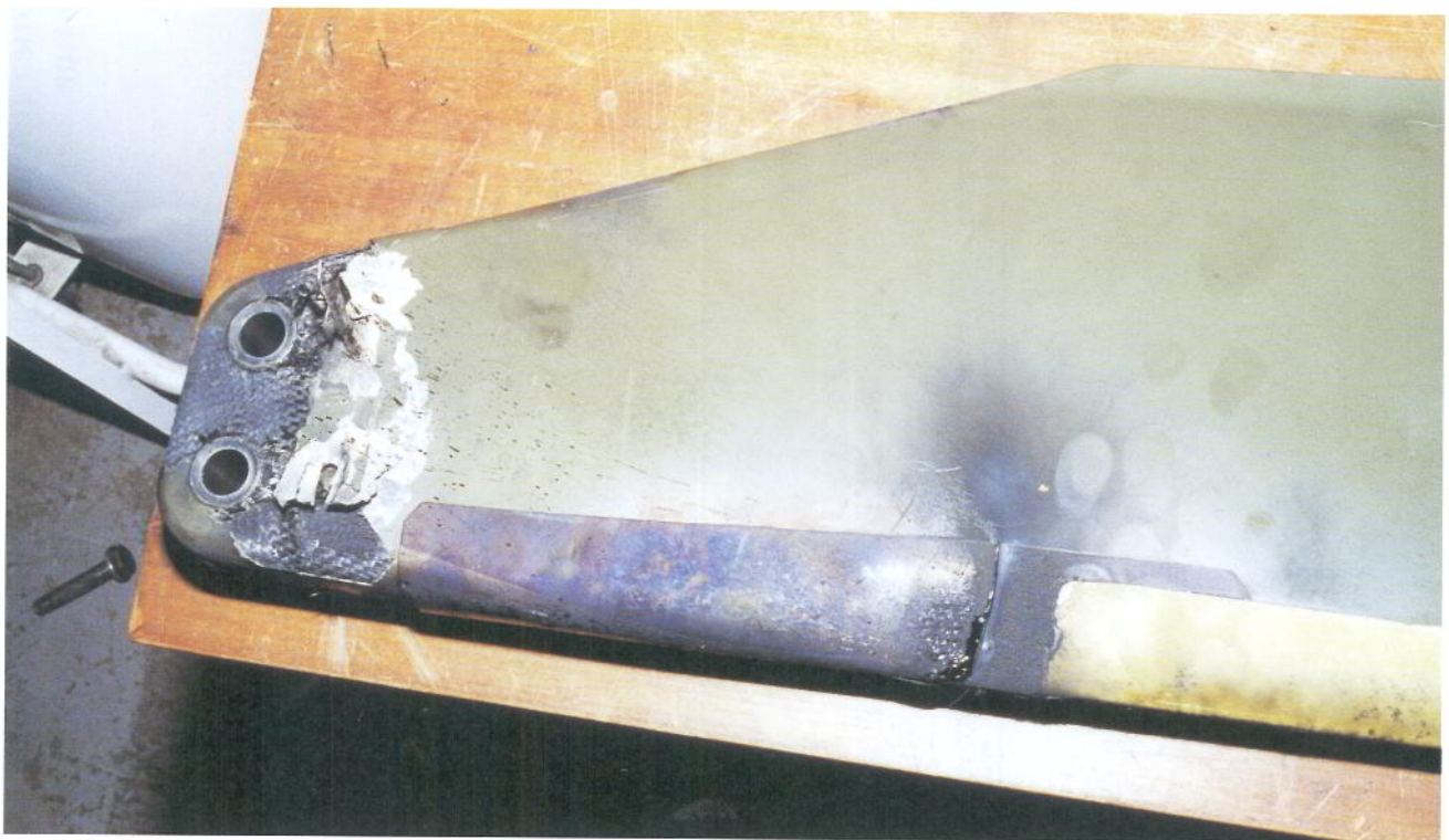
Figure 12D: Showing thermal disbonding and delamination damage to inboard side of root adjacent bushes on TRB s/n 20697.
