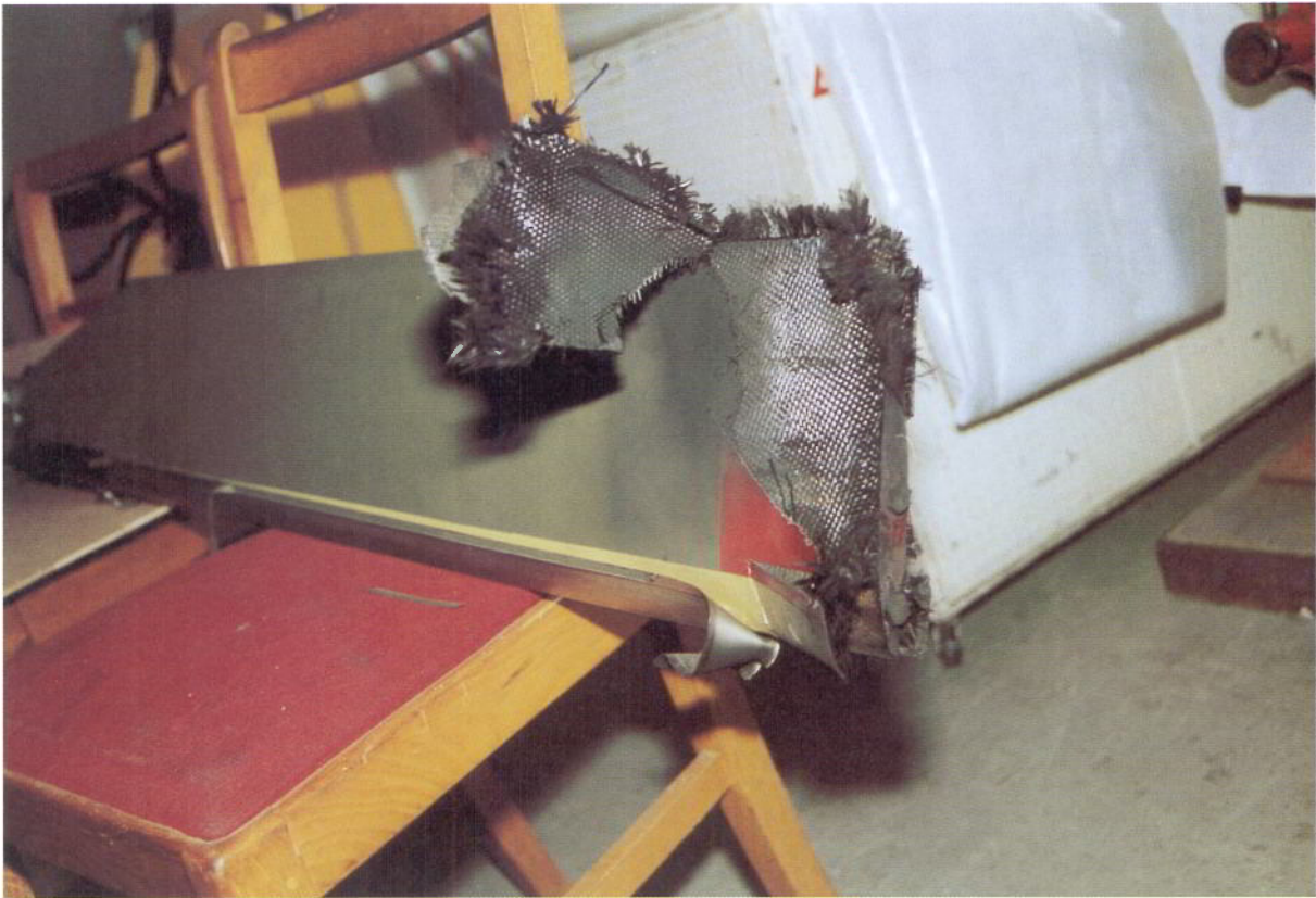
Figure 4: Showing tip damage to TRB s/n 20667 after 180.1kA input to trailing edge tip, with peel-back and general debonding of erosion shield.
