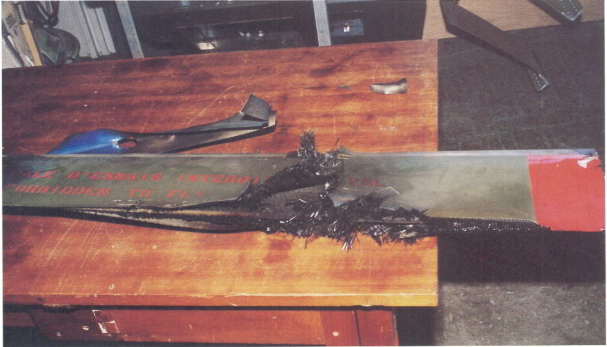
Figure 11A: Showing gross damage to aerofoil of TRB s/n 22313 after 253.3kA input to trailing edge, 34cm from tip.
