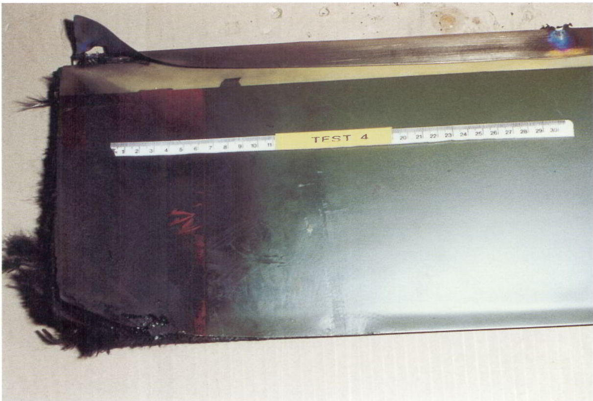
Figure 5: Showing tip damage to TRB s/n 21667 after 253.7kA input to trailing edge tip, with debonding of erosion shield and 'burn-holes'.
