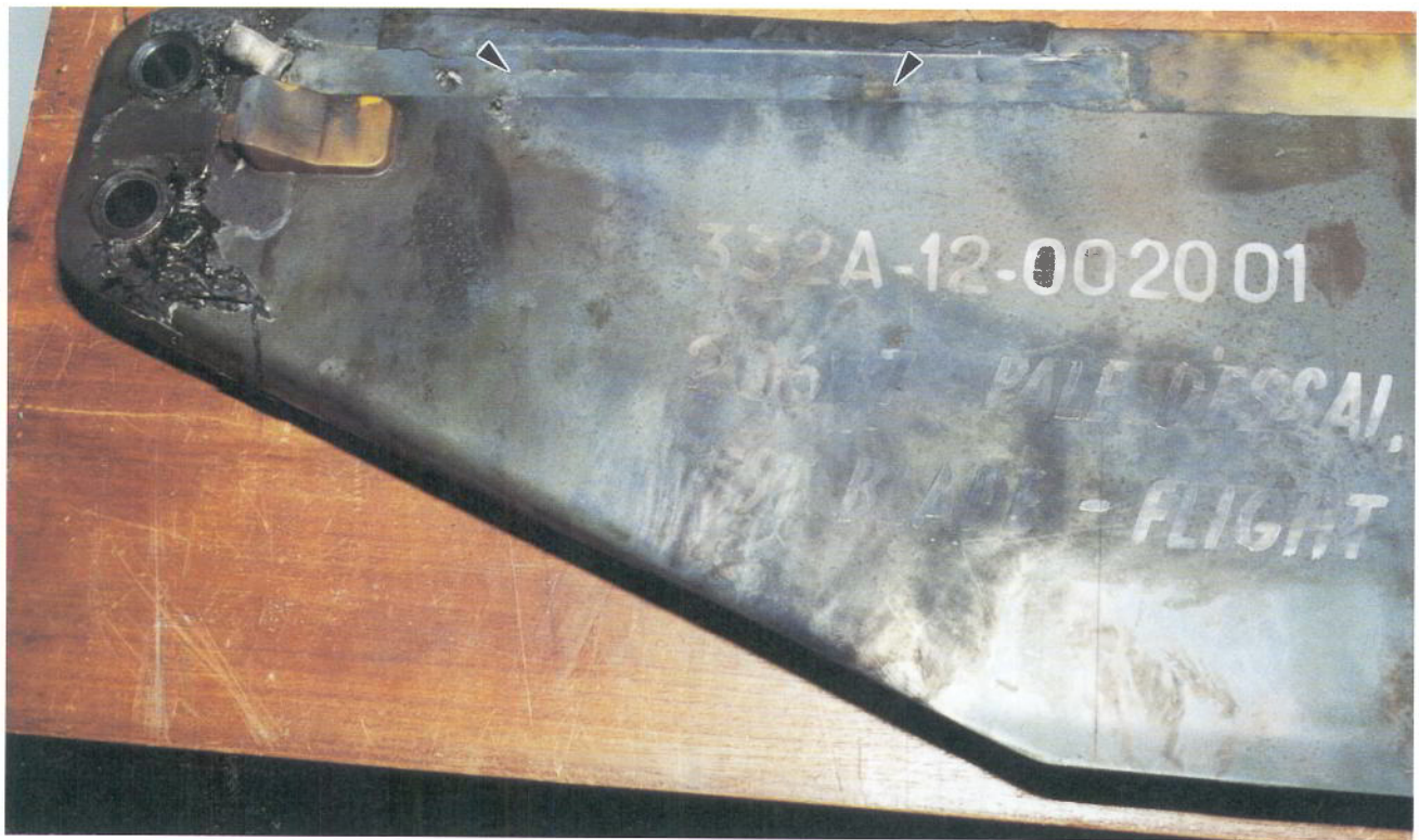
Figure 12C: Showing almost full length 'fissure'(between arrows) within substrate uncovered by loss of brass conducting strip, and root damage adjacent attachment bolt bushes on TRB s/n 20697.
