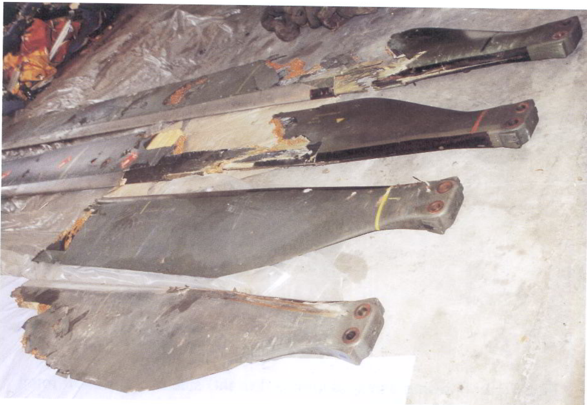
Figure 9B: Showing all recovered main rotor blade sections, with 'Blue' blade in foreground and 'Black' blade sections in background.
