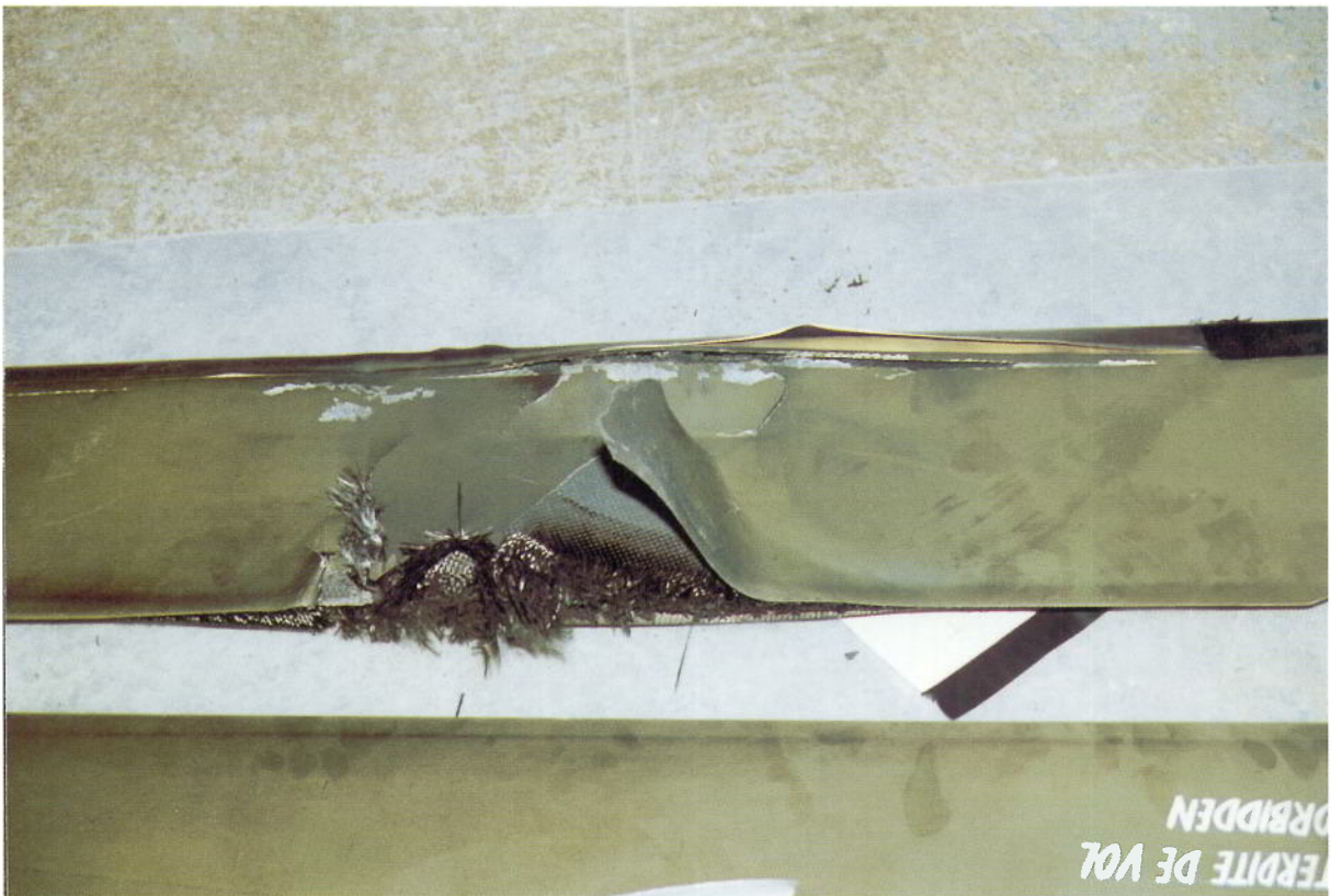
Figure 8B: Showing gross disruption of mid-aerofoil on above TRB and spanwise cracking of skins just aft of erosion shield.
