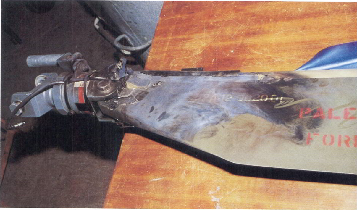
Figure 11C Showing marked thermal affects on outboard side of root on TRB s/n 22313 with carbon fibre damage adjacent attachment bolts.
