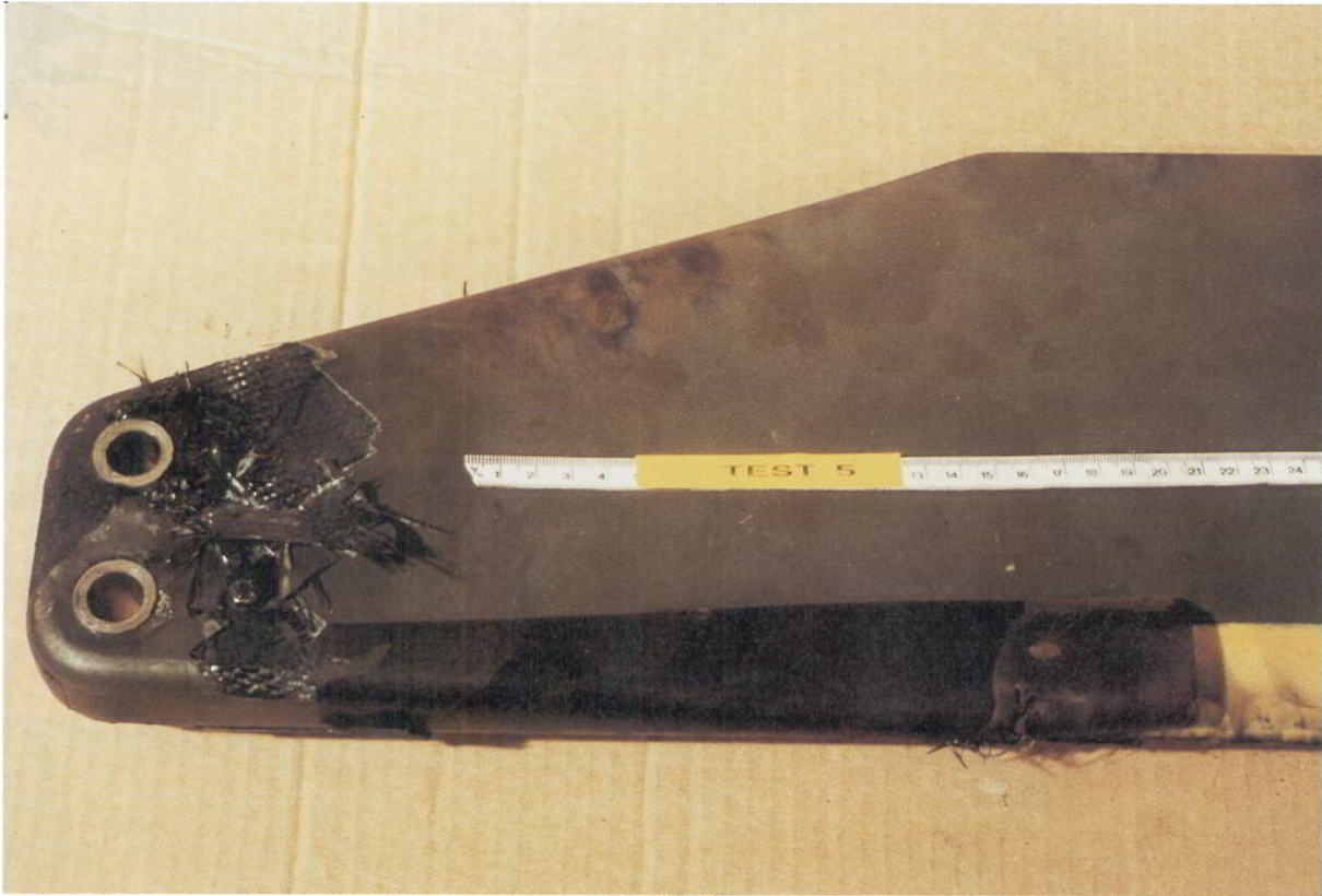
Figure 10C: Showing marked delamination and disbonding of inboard(left) surface of the root of TRB s/n 20662 after 275.5kA input to aft tip bolt.
