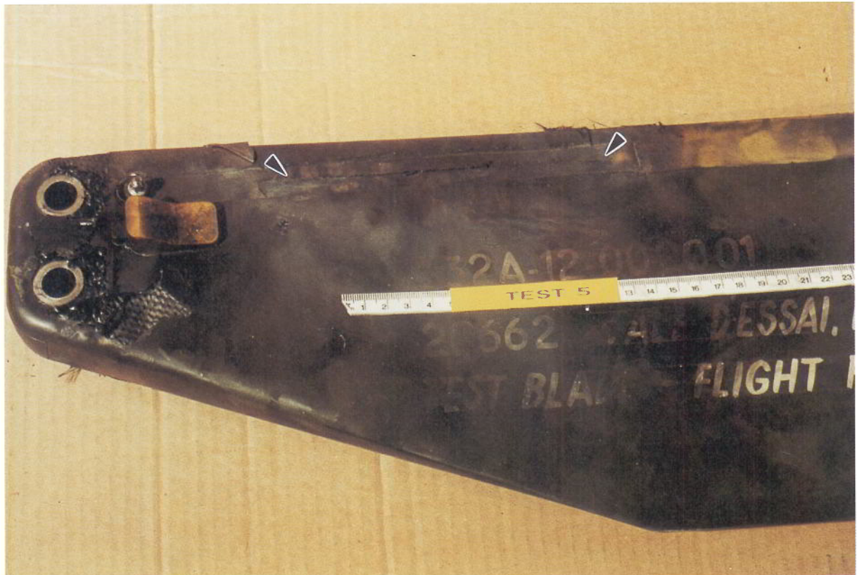
Figure 10B: Showing longitudinal 'fissure'(arrowed) within blade substrate uncovered by loss of brass bonding strip, and root damage on above TRB.
