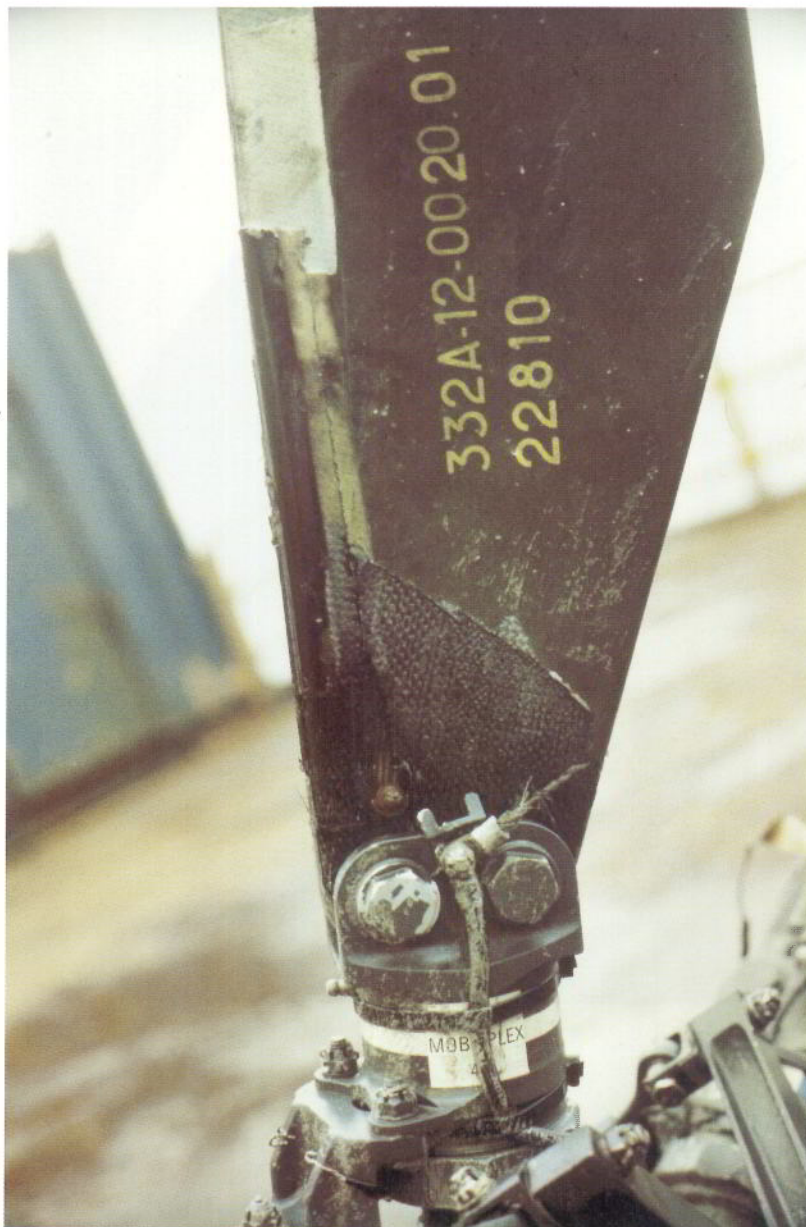
Figure 4B: Showing outboard side of 'White' tail rotor blade root with leading edge erosion shield and brass strip missing, and failed braided bonding strap.
