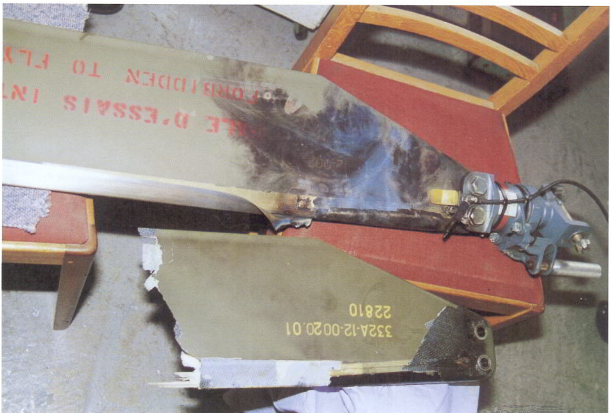
Figure 3: Showing post-test damage to inboard span of TRB s/n 22200 after 190.9kA input to shield tip, with White TRB section for comparison.
