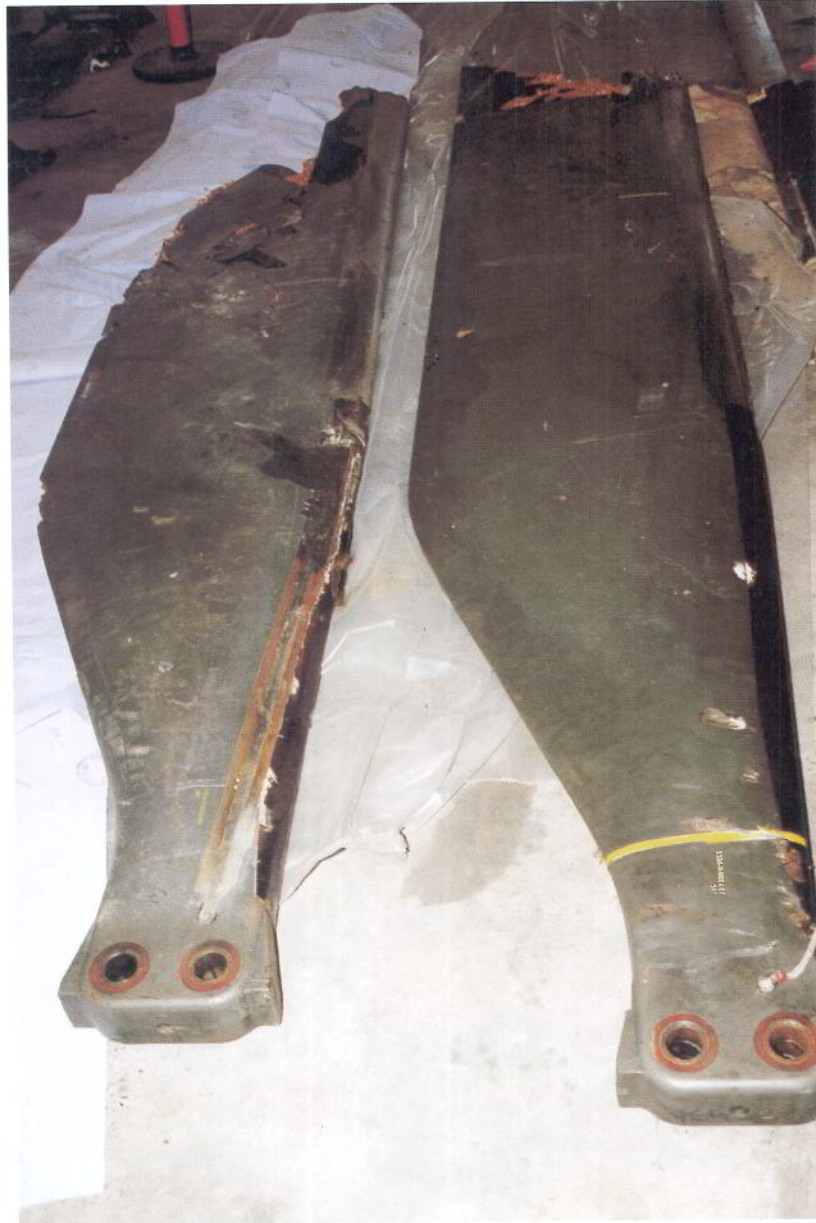
Figure 8: Showing recovered inboard section of 'Blue' main rotor blade with bonding strip missing, alongside 'Yellow' MRB for comparison.
