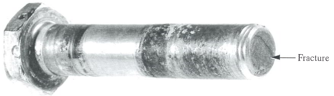
Figure 12A: Showing upper length of tail rotor gearbox upper attachment bolt with fracture face arrowed.
