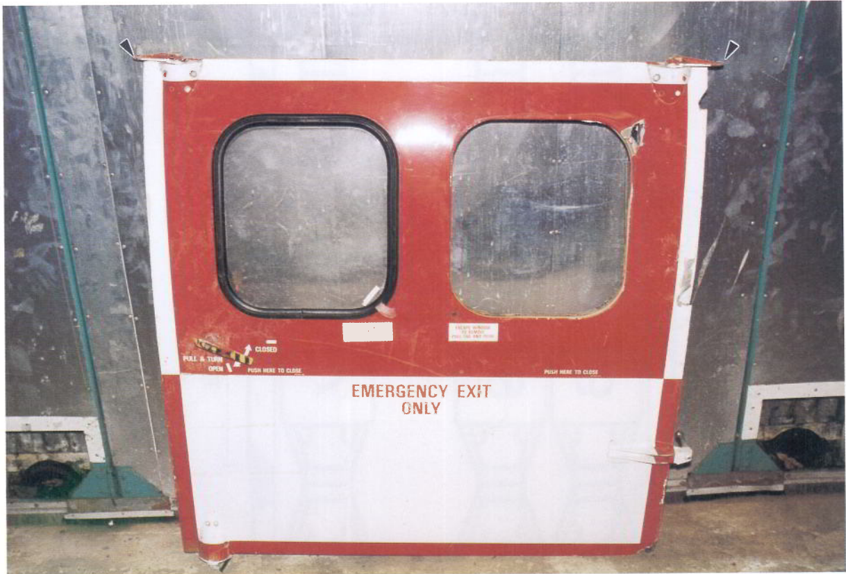
Figure 2: Showing right main door emergency exit with both spring-loaded arms arrowed.
