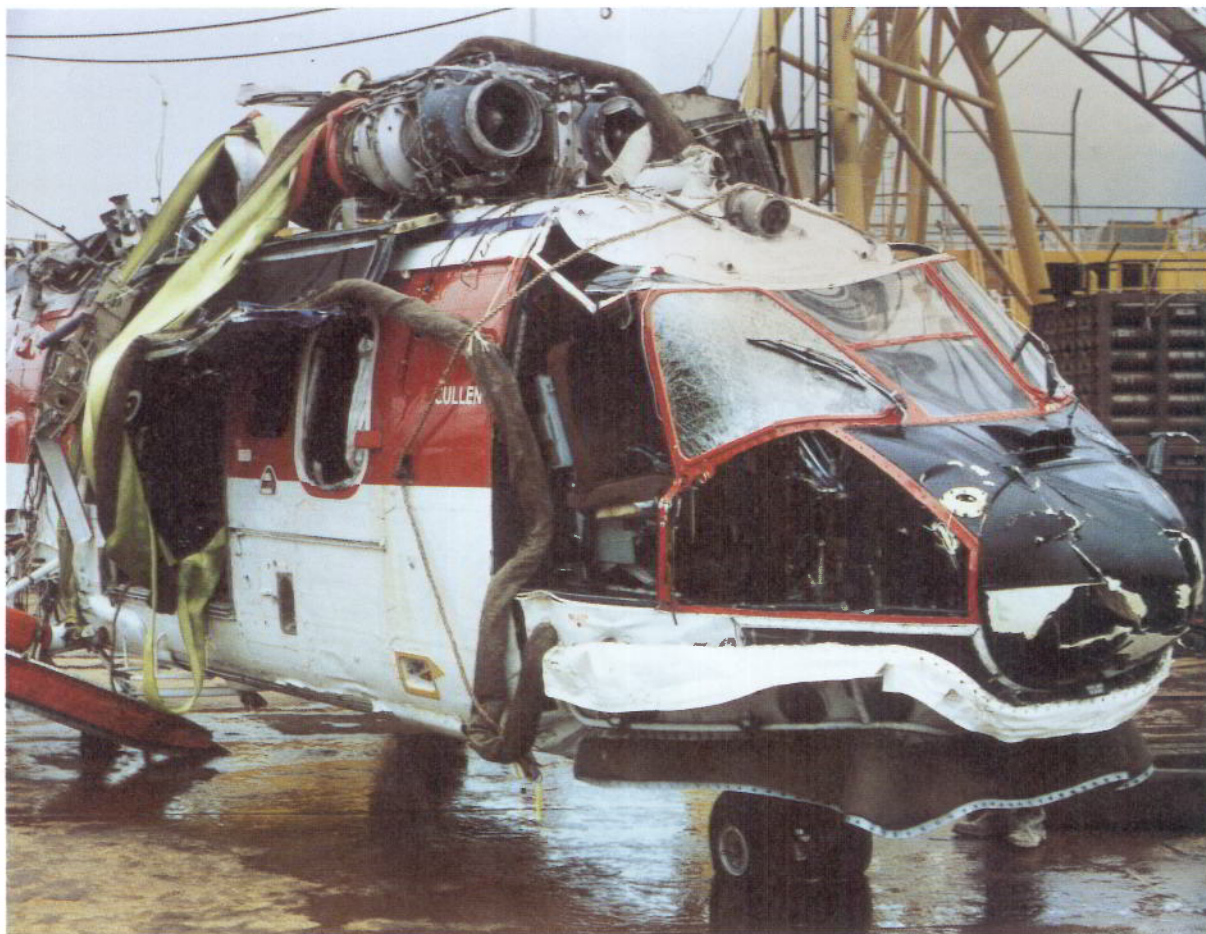
Figure 14: Showing the recovered helicopter onboard MSV Stadive without its main rotor head and main gearbox assembly which detached during the first associated 'lift' from the seabed and was recovered before the main airframe structure shown here.
