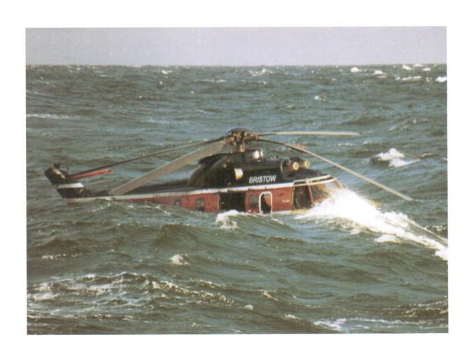
Showing G-TIGK drifting in heavy seas after ditching and evacuation of occupants, with tail rotor/gearbox missing and damaged main rotor blade.
