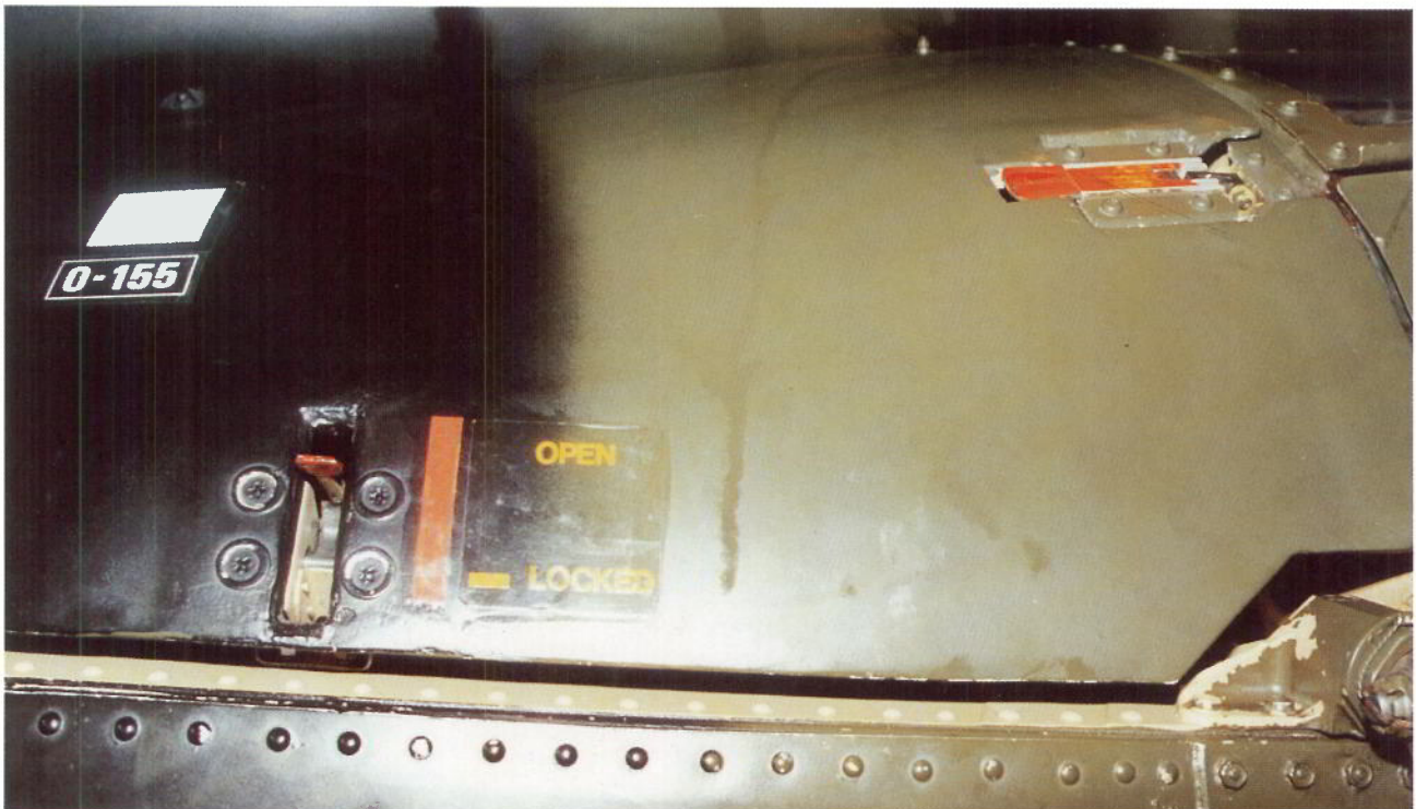
Cowling closed and latched front and rear Sprung latch not engaged
