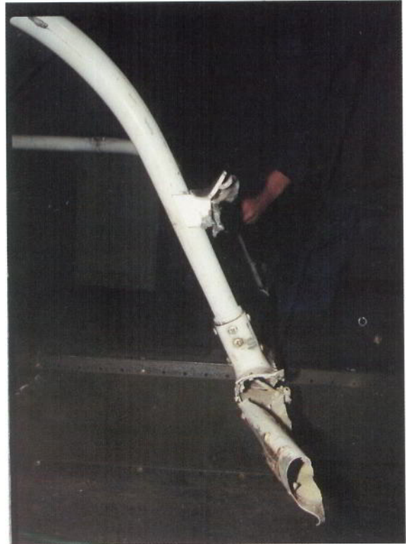
DAMAGE TO RIGHT REAR SKID OF G-BNIT, ABOVE, MADE BY MAIN ROTOR BLADE TIPS FROM G-MARC, BELOW
