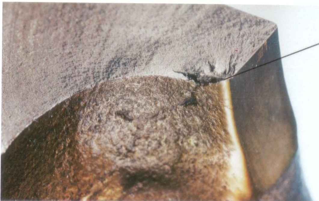
Material Defect at Connecting Rod Fracture Origin
