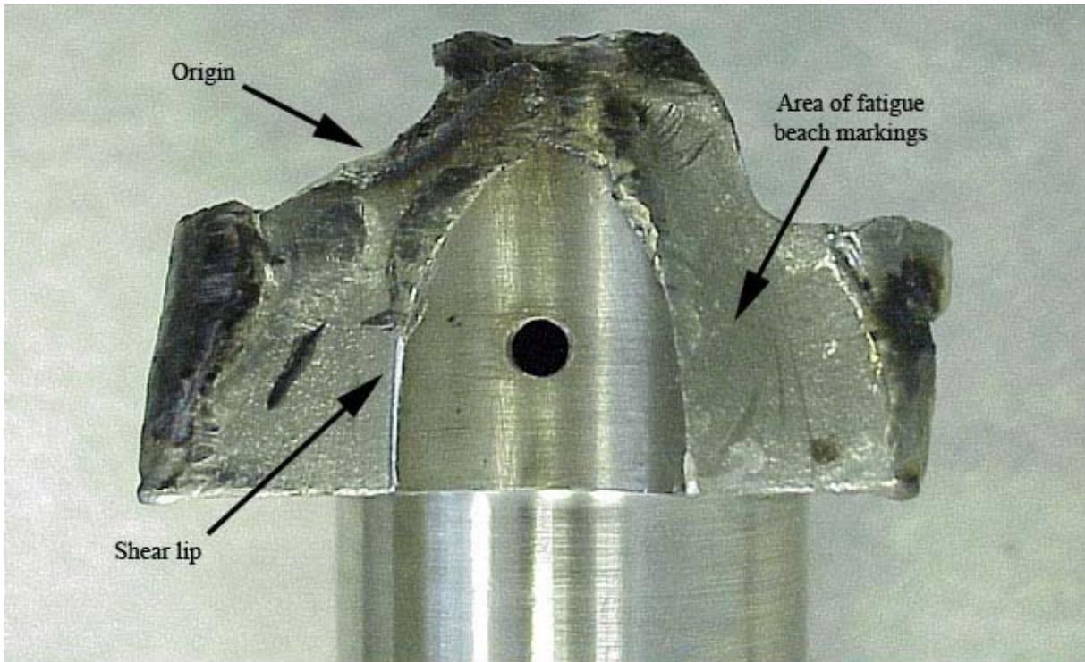
Figure 4 - Detail of crankshaft fracture surface
