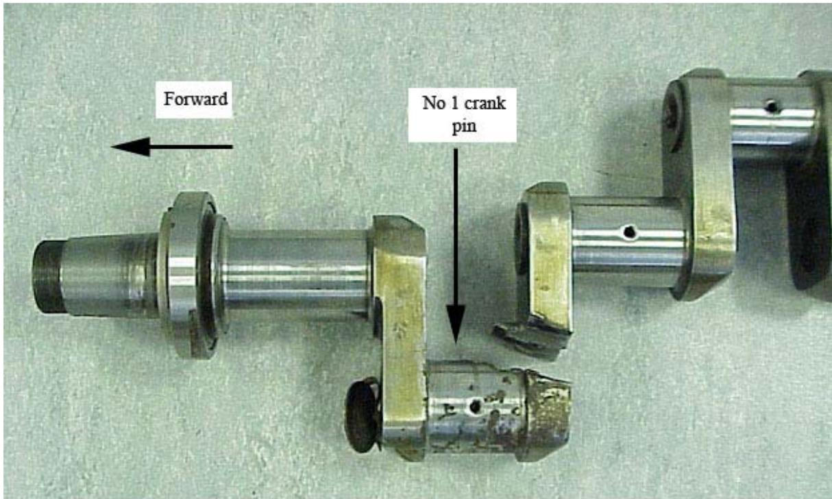
Figure 3 - Fractured crankshaft
