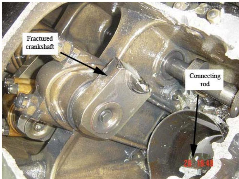
**Figure 2 - Failed crankshaft, No 1 cylinder and fractured connecting rod**
