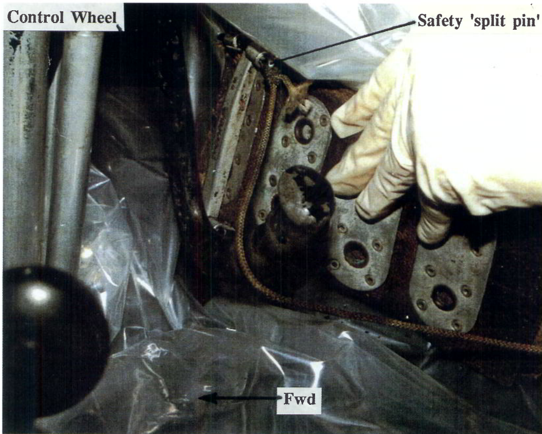
Possible snagging of control column by safety pin cord when pulled aft with left roll demanded
