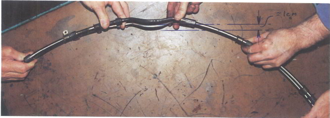
Damaged Manifold (upper) Strained into Correct Shape Above an Undamaged Item. Note difference in 'height' of Curved section Figure 4
