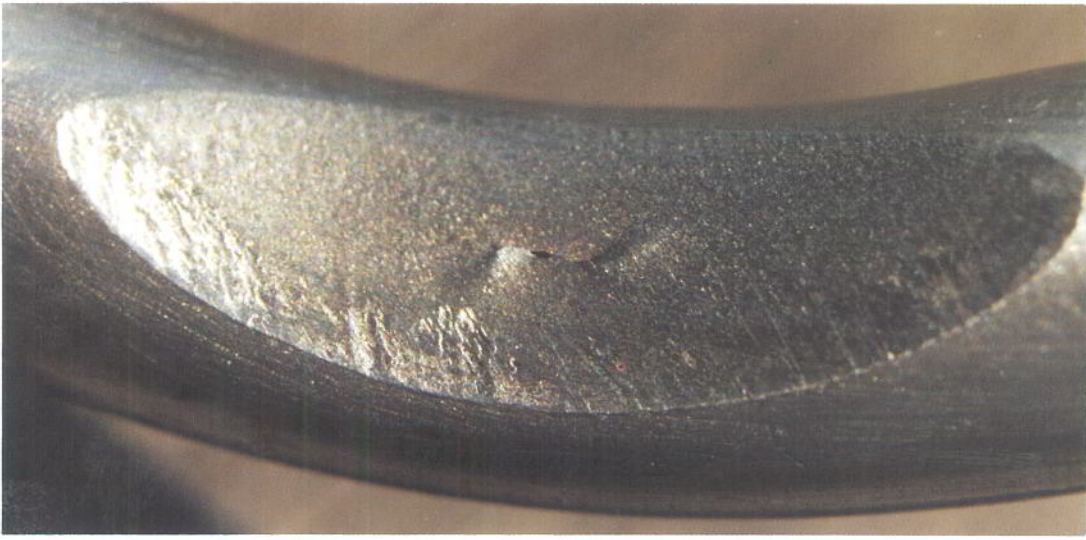
Close Up of Fuel Pipe Damaged Area Showing Central Split Figure 3
