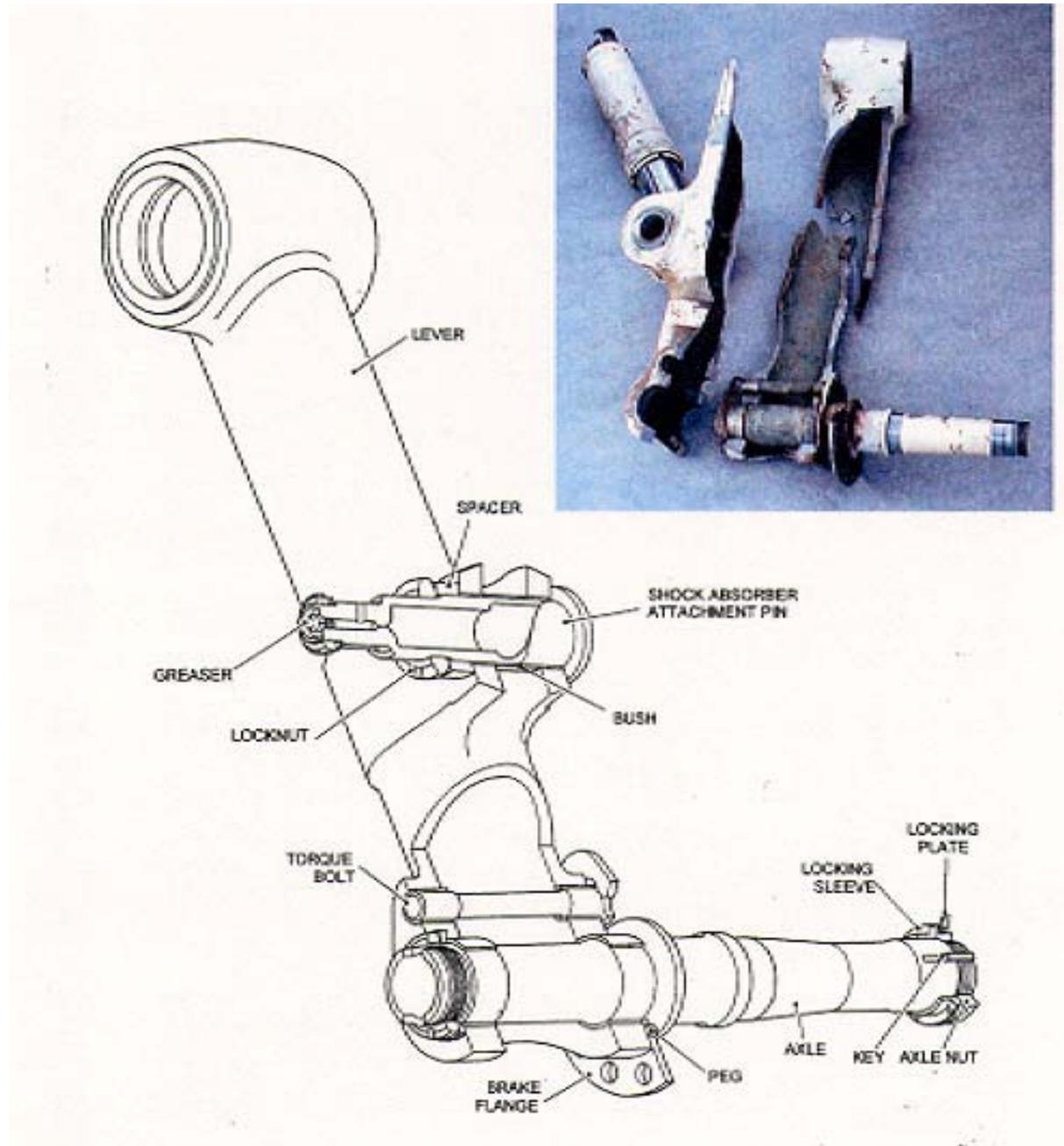
(Note: for clarity, the lever is shown sectioned at lower end. By coincidence, the failure occurred along the plane of section, as seen in the inset photograph.)
