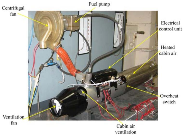
Figure 5 - Typical T310R combustion heater - bench test
