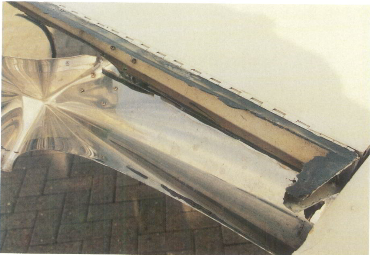
Aileron trim tab on G-TELL showing disbonding between skin, ribs and spar
