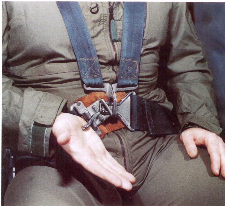
Figure 2. View of harness with buckle in potentially jammed position (Photo: RAF School of Aviation Medicine)
