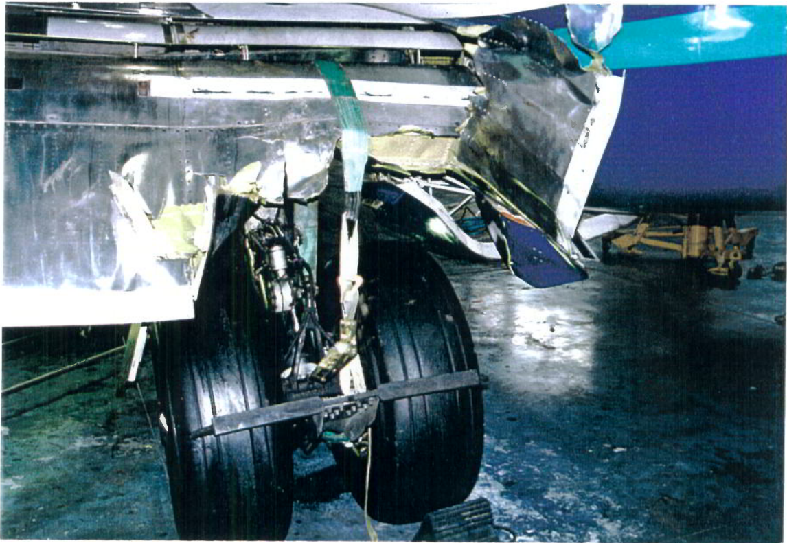
G-DEVR on jacks post-accident. View of left MLG from aft looking forward showing damage to trailing edge flaps
