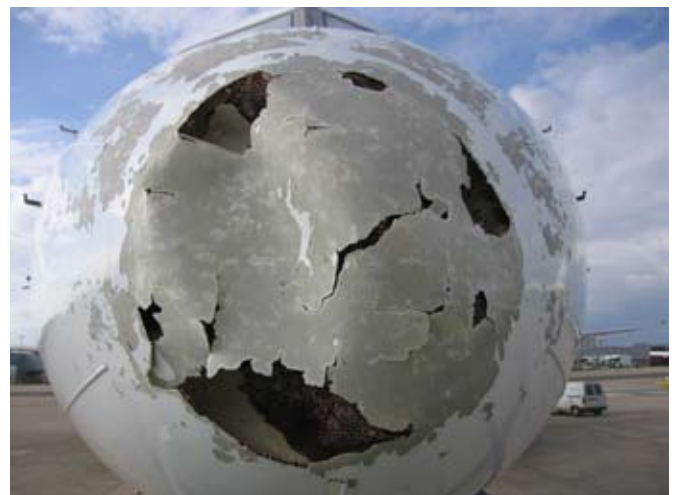
Figure 1 Damage to radome
