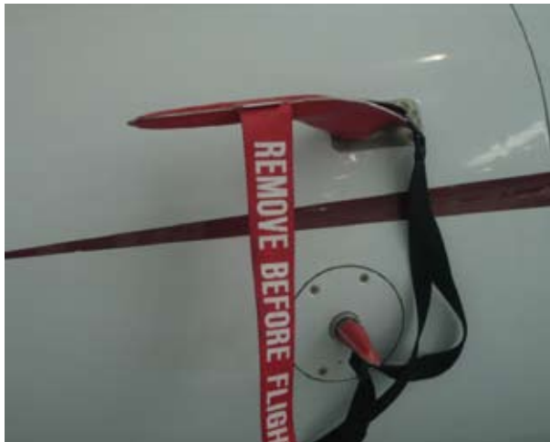
Left pitot probe and AOA vane below Standard cover
