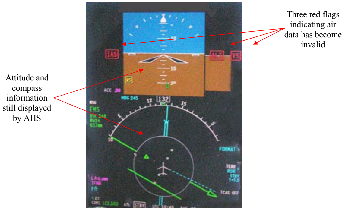
Figure 3 PFD display with air data information invalid
