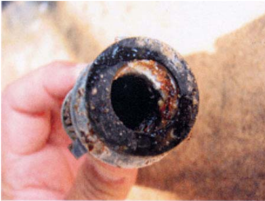
Figure 2: Corrosion on fuel filter element
