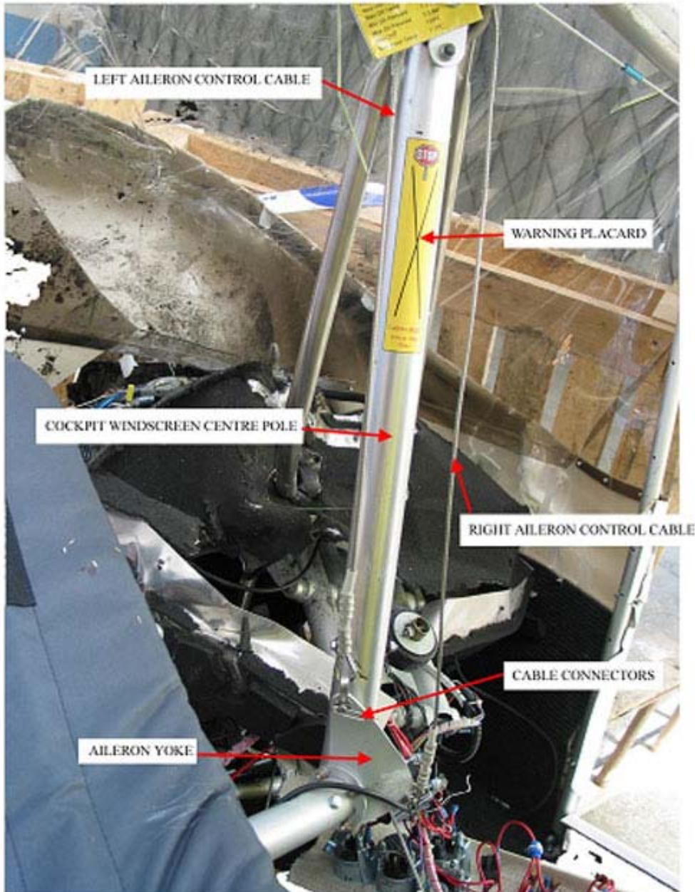
**Aileron control cables cross connected to the aileron yoke on the accident aircraft**
