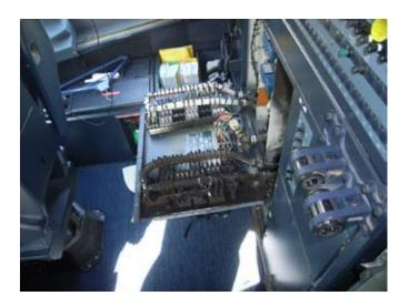
**Figure 4**General view of damage to panel 123VU
