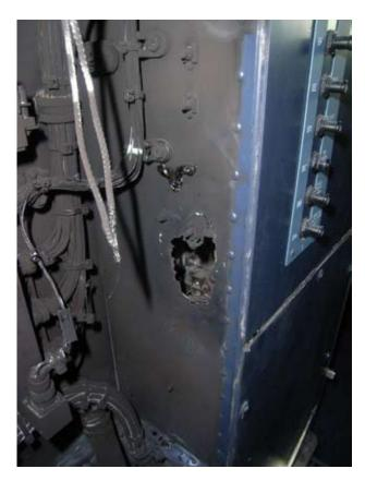
**Figure 6**Structural damage outboard of panel 123VU
