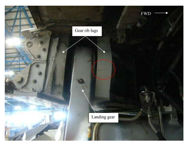
**Figure 4** Landing gear support rib with cracked forward lug
