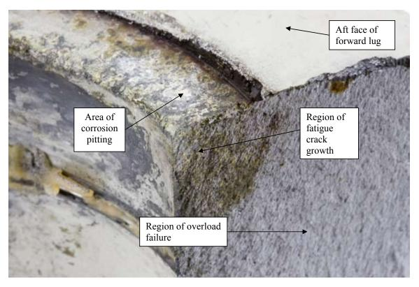
Figure 7 Detailed view of forward lug fracture surface
