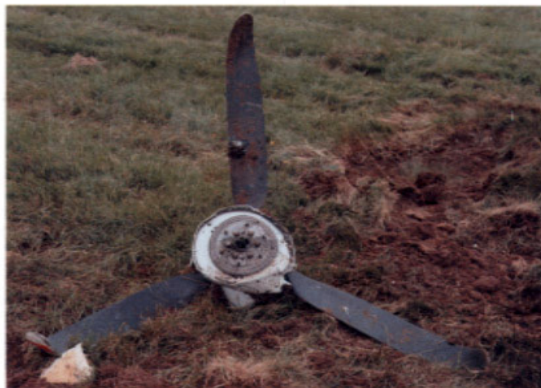
Figure 2 - Photograph of right propeller as-found. Note curled tips to blades.
