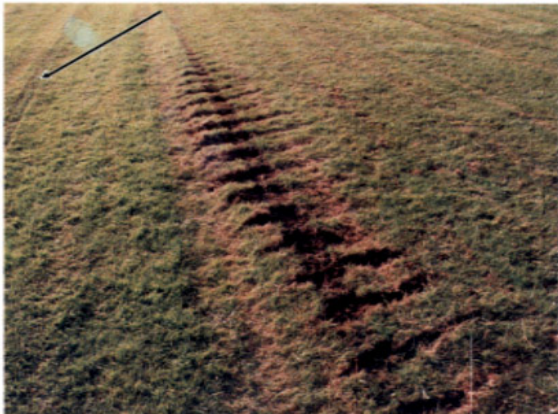
Figure 1 - Photograph of wheel marks and propeller slashes looking in the take-off direction. Note impression of nosewheel tyre (arrowed)
