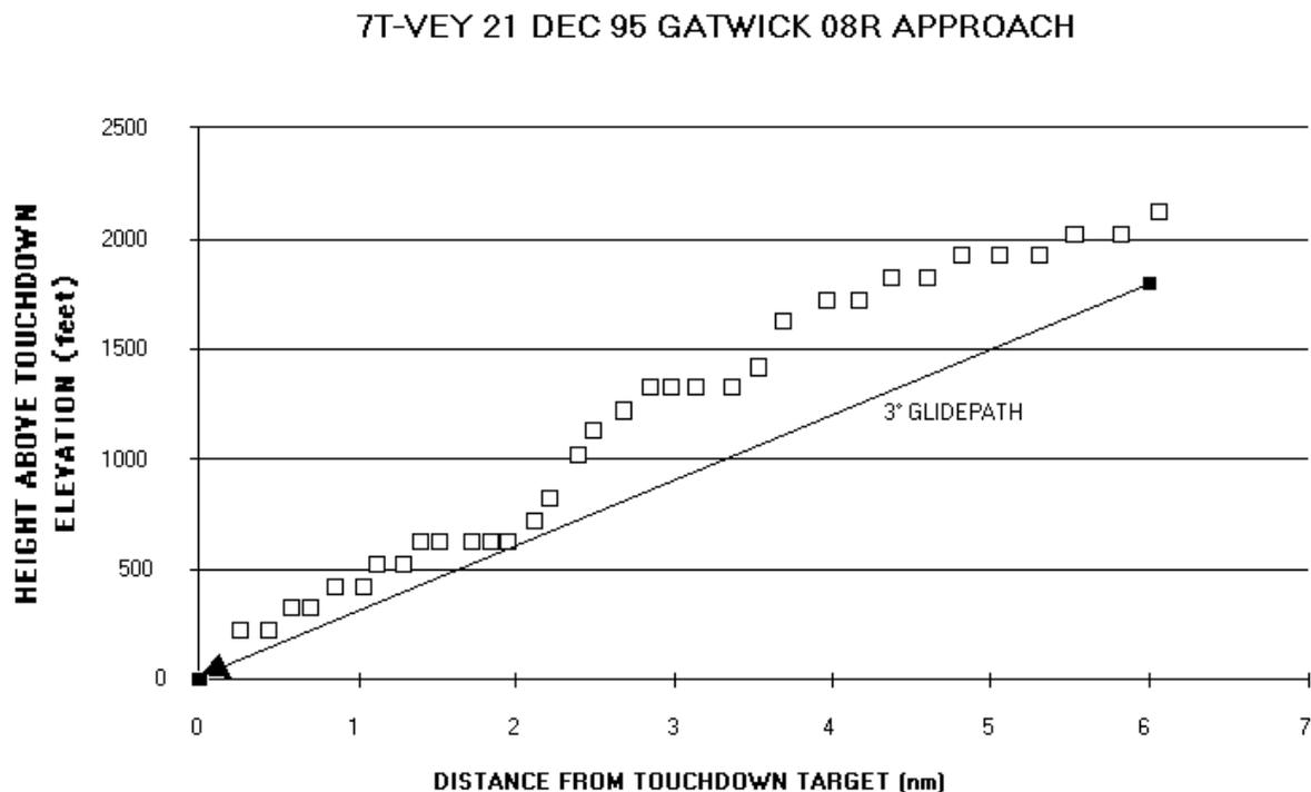
The maximum rate of descent, some 2,100 feet per minute, was achieved just outside 2 nm from the touchdown target. With the Mark 1 GPWS system fitted to this aircraft, the only aural alert available for Mode 1 (Excessive Descent Rate) was "WHOOOP WHOOOP PULL UP". On the later standard of GPWS fitted to the Boeing 737 series, this rate of descent would have triggered only a "SINK RATE" aural warning at this height above the ground.
