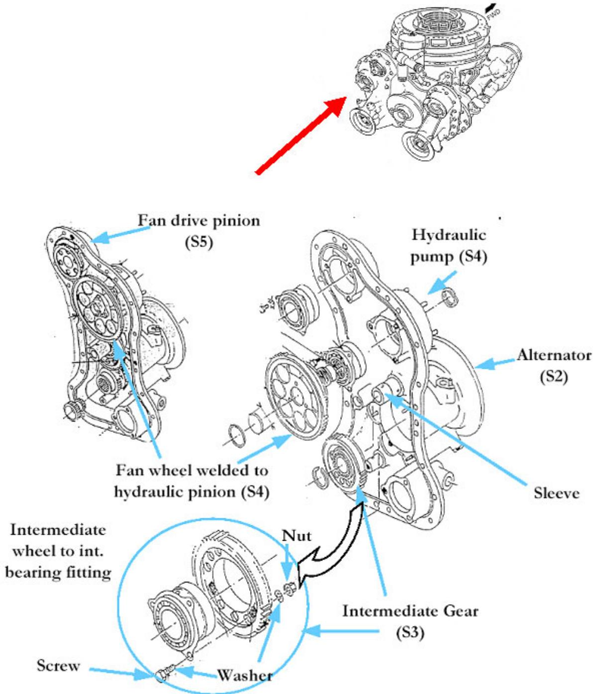
**Figure 1 Details of left hand accessory module**
