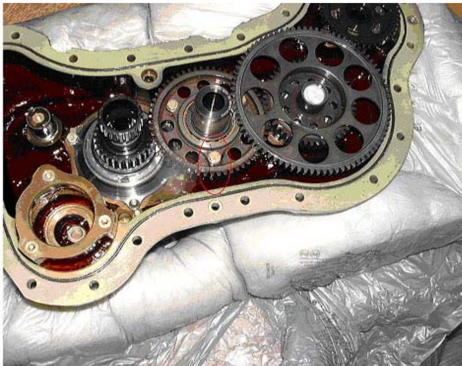
**Figure 2 LH accessory gearbox from G-JSAR, showing cracked intermediate gear**
