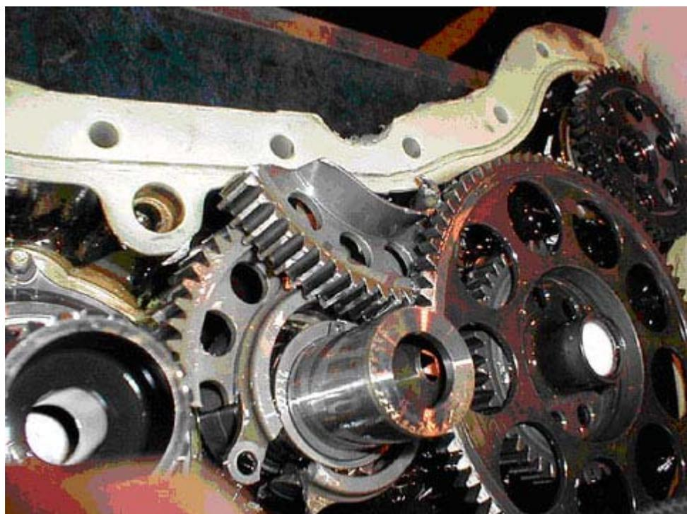
**Figure 3 Failed intermediate gear from G-PUMS**
