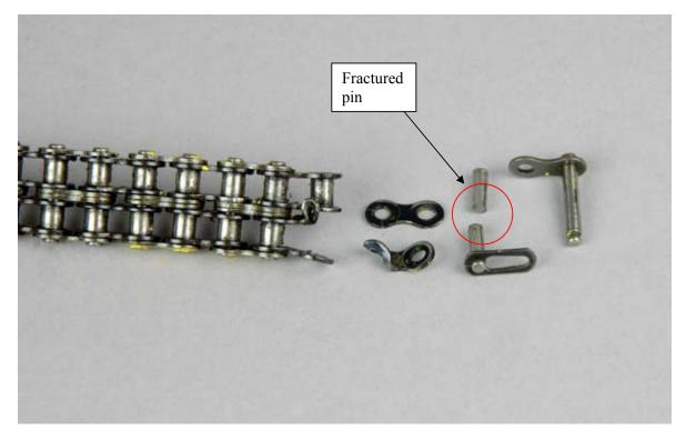
**Figure 1** Failed chain link
