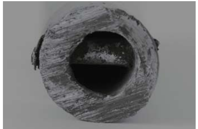
Figure 6 Detail of failed scroll pin in pivot shaft
