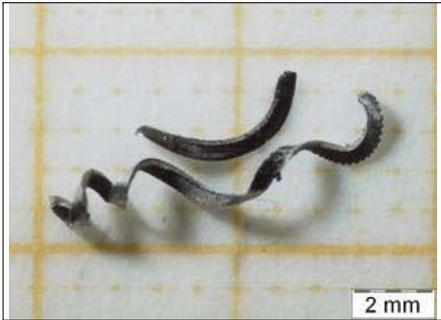
g) Particles from abrasion or wear
