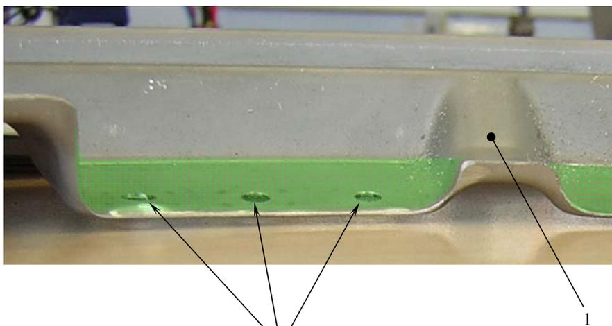
Clearance holes for the attachment rivets (g) for the magnetic elements (e)
