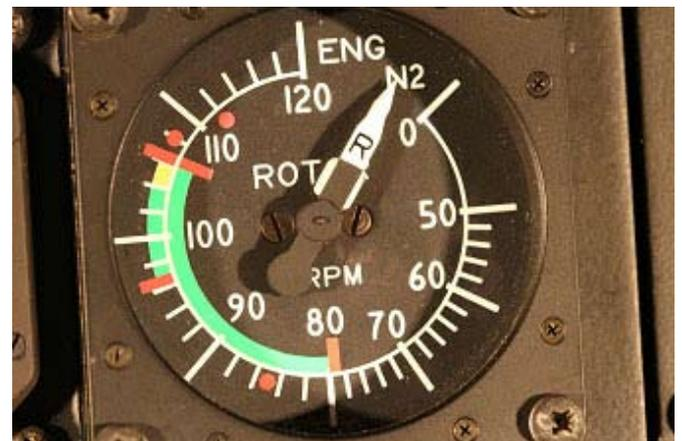
The two N2 pointers are below the NR pointer in this photograph of the gauge at rest.
