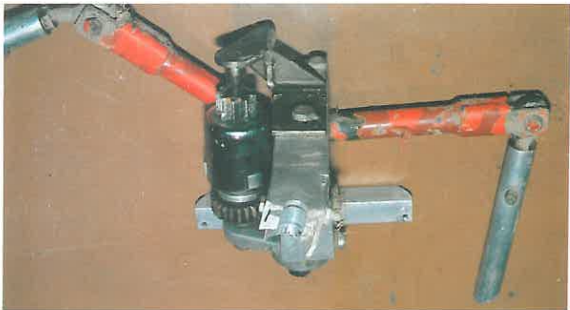
VIEWS OF TORQUE TUBE SHOWING FAILURE AND DISTORTION OF AFT SECTION
