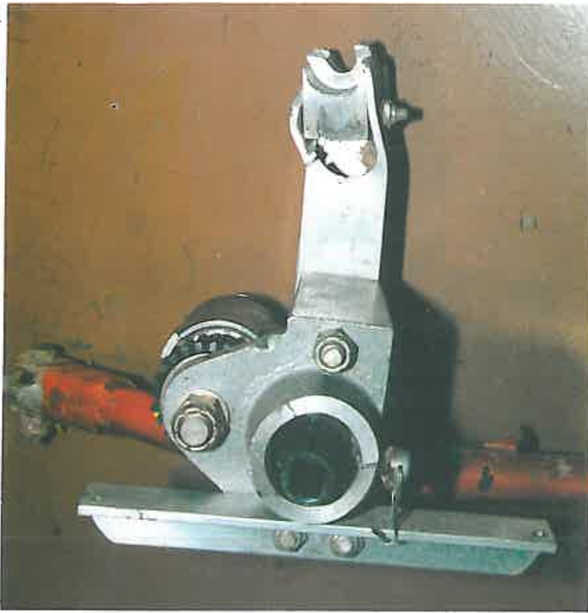
VIEW OF UNDERSIDE – SHOWING DAMAGE TO SOCKET
