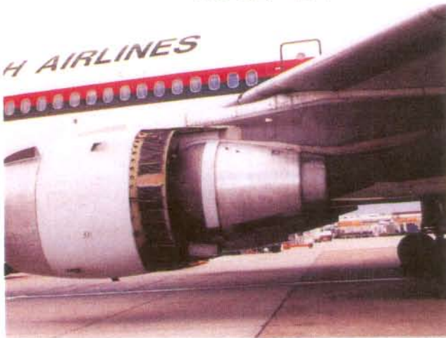
FIG 1 CF6-50/-45 THRUST REVERSER SYSTEM
