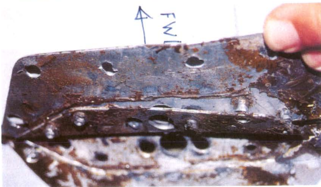
FIG 5 View of repair, with patch plate and "packing piece" being removed from cowl
