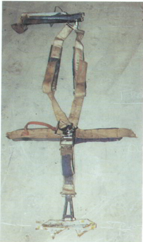
Complete Harness Showing Failures of Structural Members
