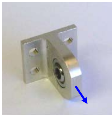
Type 2 - 7mm lug mounted on the tailplane with screw fixings
