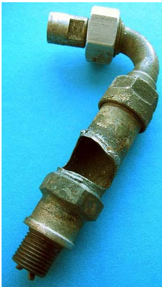
View of damaged spark plug showing burn through and empty core
