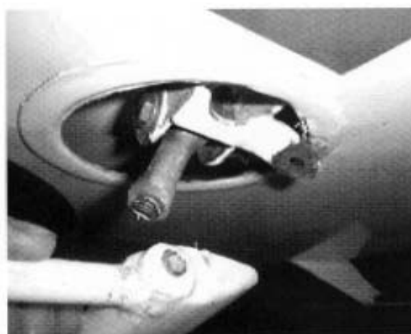
Figure 5 Fractured left wing aft strut
