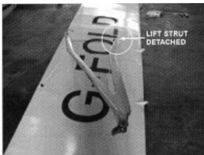
Figure 3 Buckled Left Wing Struts (aft strut has detached at wing end)
