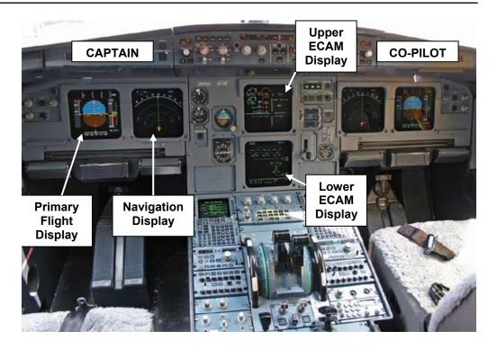
Figure 1 Electronic Flight Instrument System
