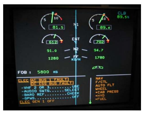
**Figure 2** ECAM Engine/Warning Display
