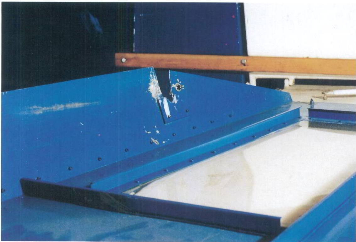
G-BPKK rear window assembly incorporating flapperon torque tube bearing half with evidence of rough trimming and mis-shapen profile
