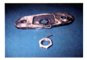
There was normally no maintenance requirement to disturb the outboard attachment area of this vane and, during checks, only routine visual inspections would have been conducted. In March of 2002, a Special Inspection to check for cracks in the flap vane 'Tee' fittings (see Figure 1) would have required this area to be dismantled. The last major work input associated with this area was during a 'C' check, carried out in July 2002, when this area was inspected but not disturbed.
