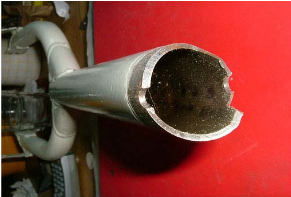
Figure 1. Lower section of failed nose gear. Note the bolt hole orientation
