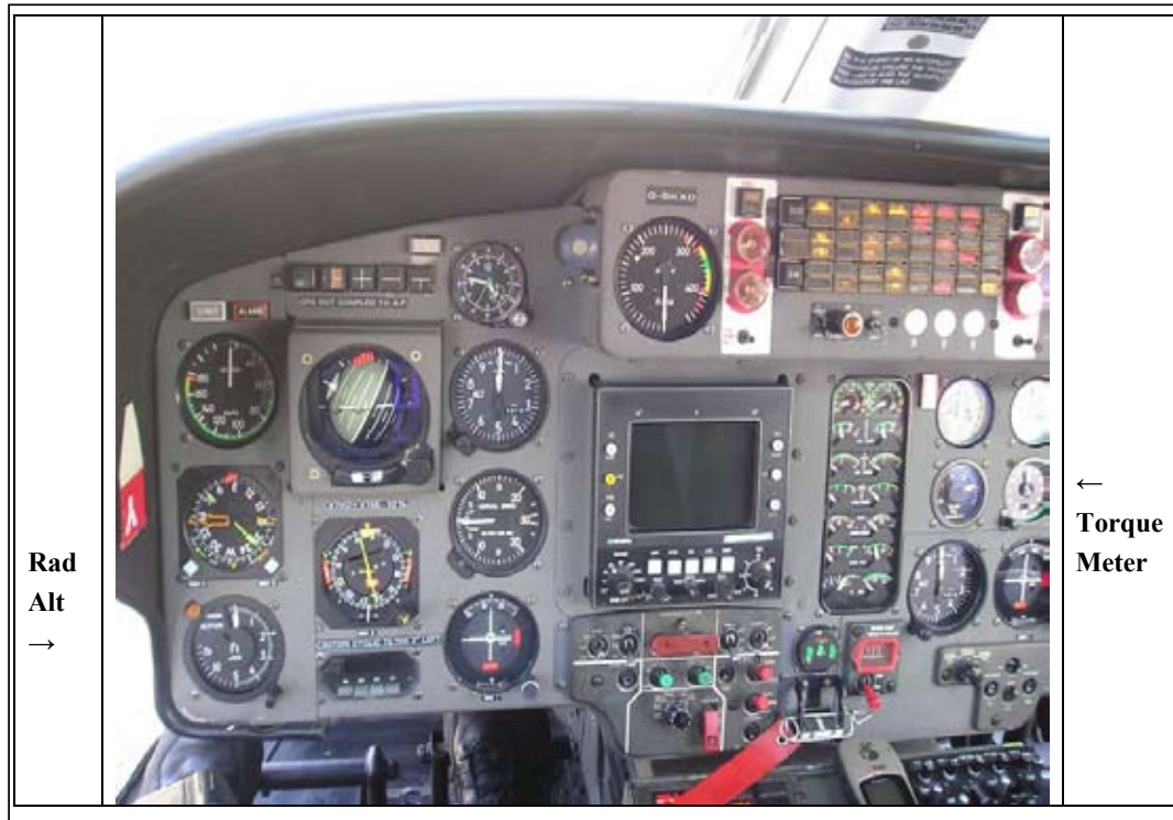
Fig 2. The LHS Panel and position of the torquemeter
