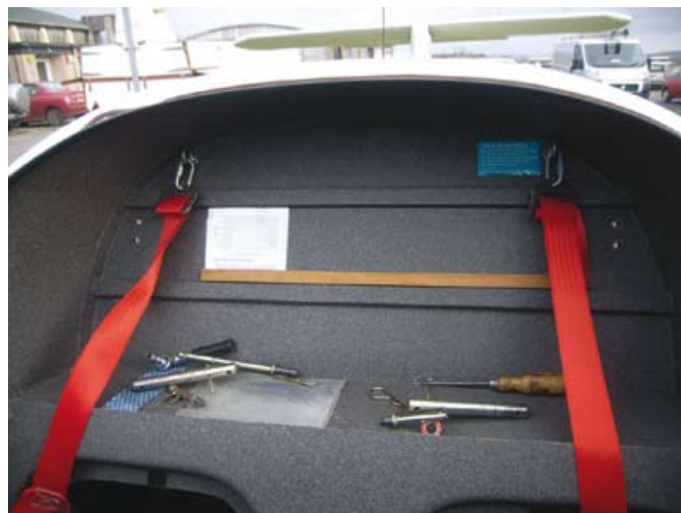
Figure 4 Shoulder harness installation
