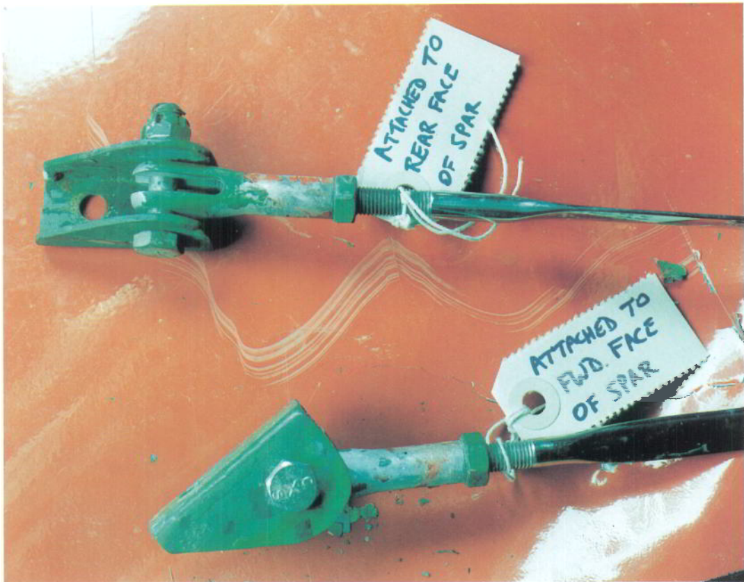
FIGURE 2. Right hand front flying wire attachments; as found
