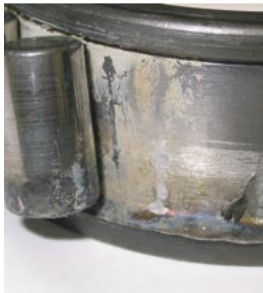
Figure 7 (right) Distortion of cone large rib face
