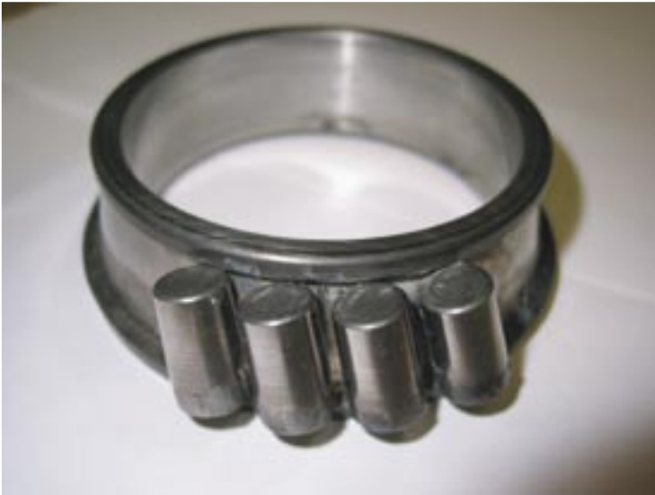
Figure 6 (left) Rollers welded to cone
