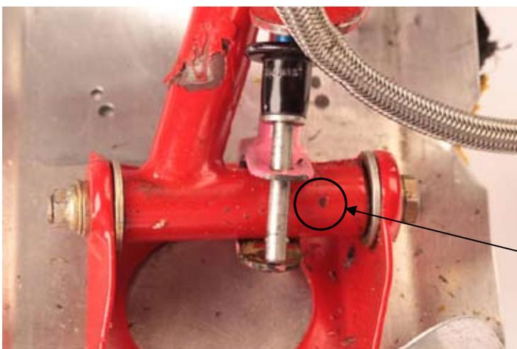
Note the witness mark on the pivot tube probably made by the pip-pin.
