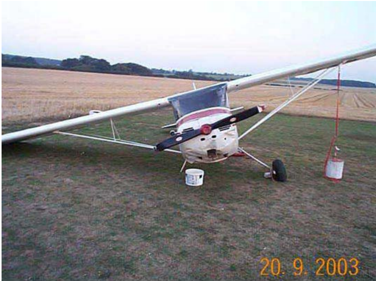
Figure 1 - Failure of right gear leg on G-BRJC
