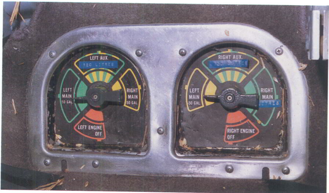
Fuel Selector Valve Levers set horizontally in Cockpit Floor between Pilot's Seats
