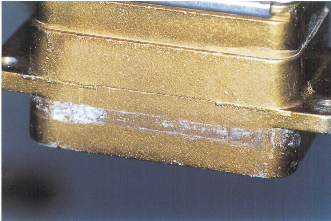
View of YDC connector shell showing evidence of dry corrosion products on exterior surface
