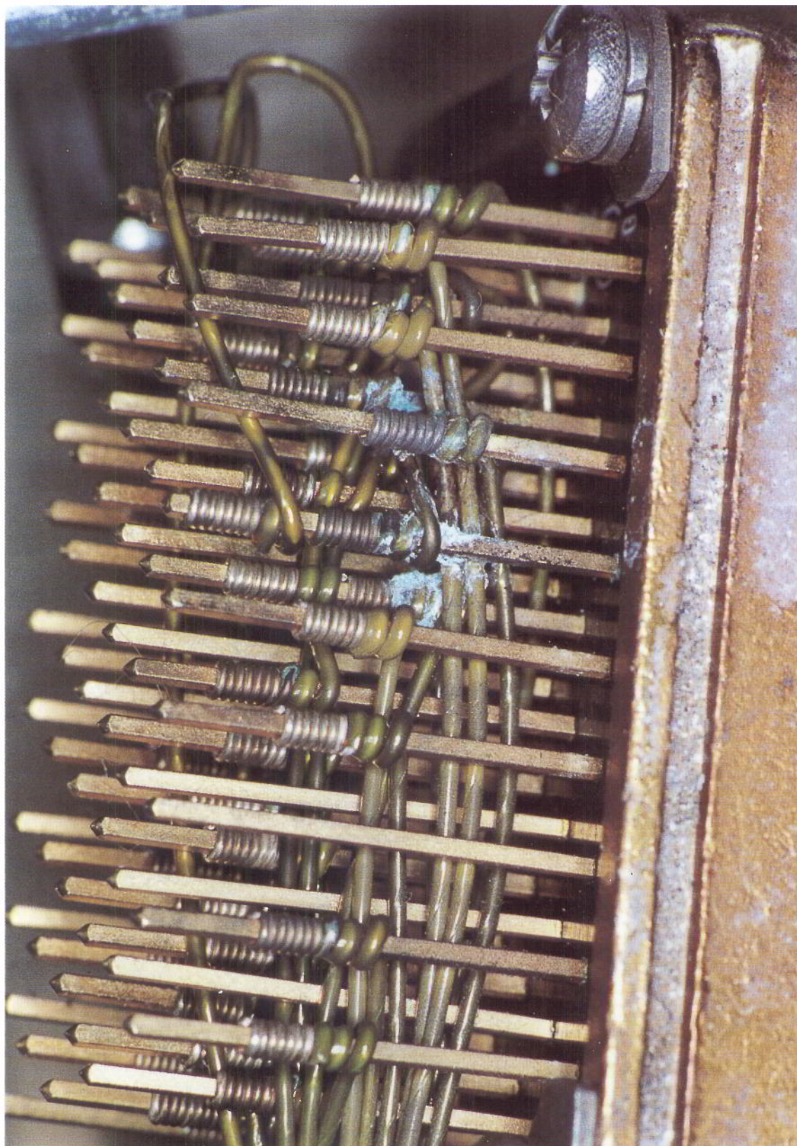
Close-up view of terminal posts at the back of Yaw Damper Coupler connector showing accumulation of electrolytic/corrosion deposits around wire-wrapped joints
